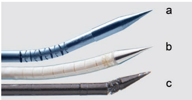
Figure 1.2. Examples of steerable needle prototypes – a) a steerable needle with stainless steel segments, b) an MRI compatible steerable needle, and c) a needle with a steerable tip positioned on top of a miniature ball joint. [all prototypes designed and fabricated in the MISIT lab of the Delft University of Technology, The Netherlands].
