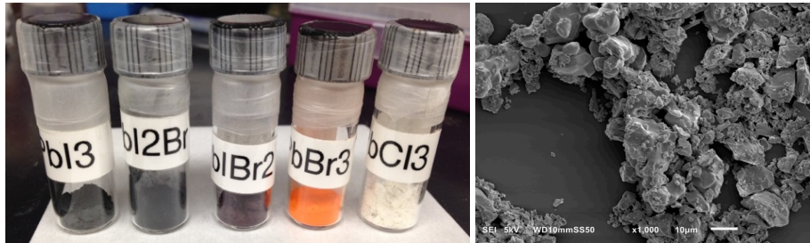
Figure A3.1 \text{CH}_3\text{NH}_3\text{PbX}_3 ( X = \text{I}, \text{Br}, \text{Cl} ) powder materials. Left) Camera image. Right) SEM image of polycrystalline micrometer crystals of \text{MAPbI}_3 .
