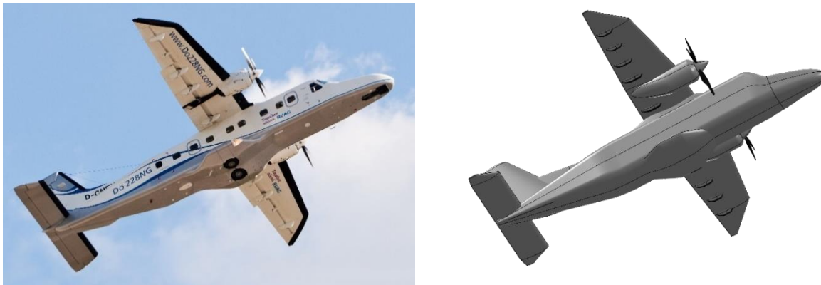
Fig. 1 Comparison between Do 228NG [14] (left) and the 19-seat baseline aircraft (right).
