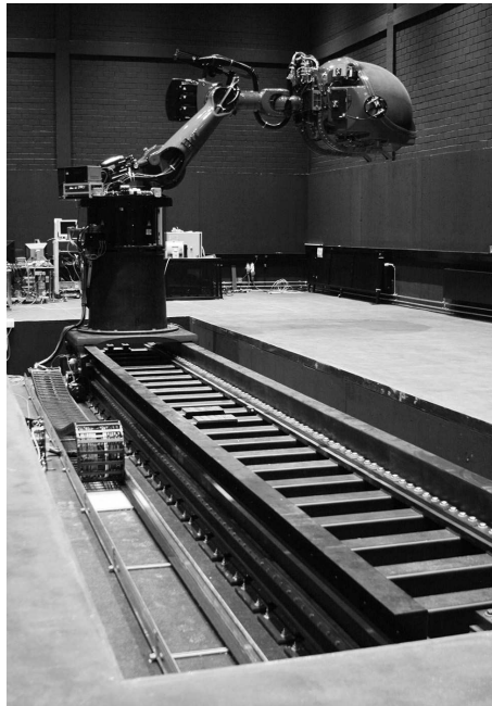
Figure 3.10: The MPI CyberMotion Simulator on a linear axis and with the enclosed pilot station at the end of the anthropomorphic robot arm.
