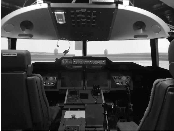
Figure 3.14: Interior of the SRS, showing the projected visuals, instruments and CLS-driven helicopter controls.
