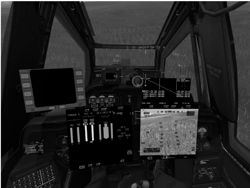
Figure 4.11: Illustration of virtual cockpit instruments and HDU overlay in the VR-enabled visual environment of the Desdemona simulator.
