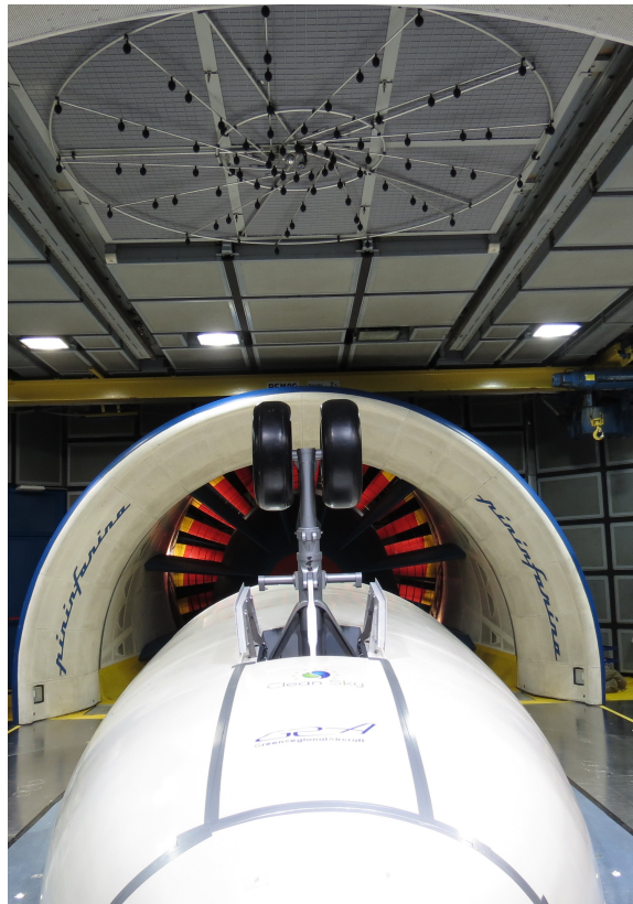
Fig. 2: ALLEGRA NLG model inside the wind tunnel with the top array visible [49].
