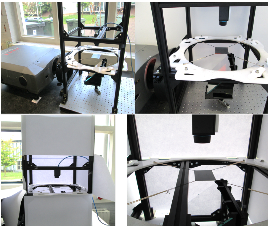
Figure 7.2: Picture of the developed setup. The setup is surrounded by white paper to block the air flow from an air conditioner in the laboratory.
