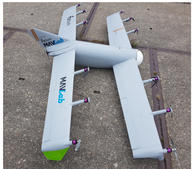
Fig. 1. NederDrone2 with 12 propellers of which 8 are foldable and stop during forward flight. The 4 tip propellers remain active during forward flight and have a higher pitch for efficient fast flight. The large fuselage can accommodate a 9 liter pressure tank and a fuel-cell.
