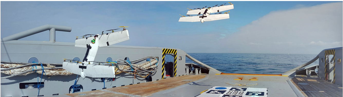
Fig. 10. A composite photo from a NederDrone 1 prototype in hover and subsequently in forward flight, operated from a ship on the North Sea.
