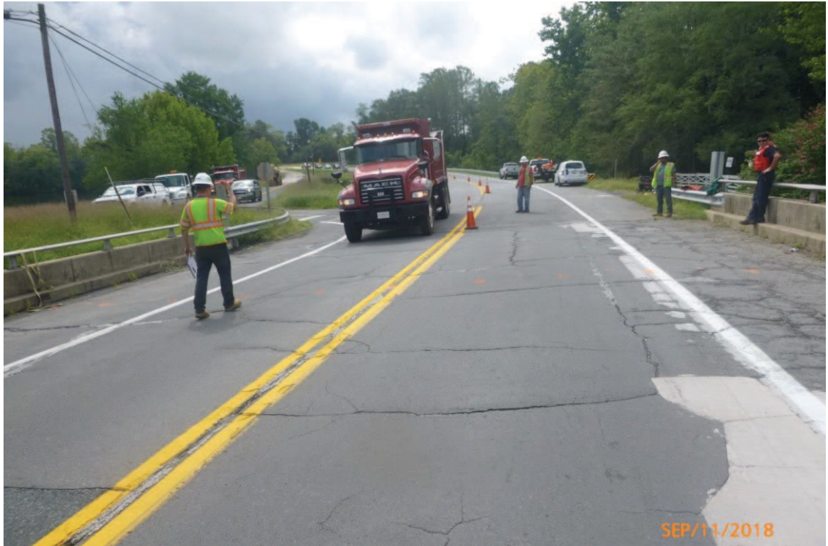
Figure 2. Proof load test on bridge with cracks in overlay along joints of the box beams
