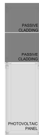
FIG. 9 Front view of the PV macro-panel hosting a top passive cladding. The PV panel frame is mechanically fixed to the removable façade fixing system (as per the passive claddings) thanks to rivets.
