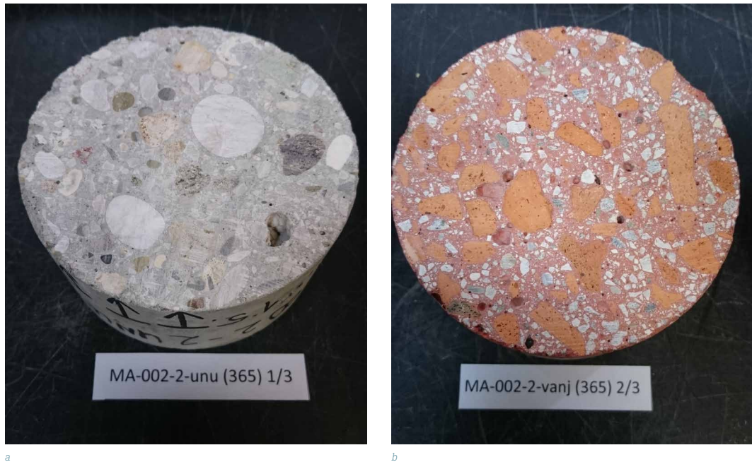
FIG. 2 Recycled aggregate concrete: a) old crushed concrete as recycled aggregate; b) crushed brick as recycled aggregate
