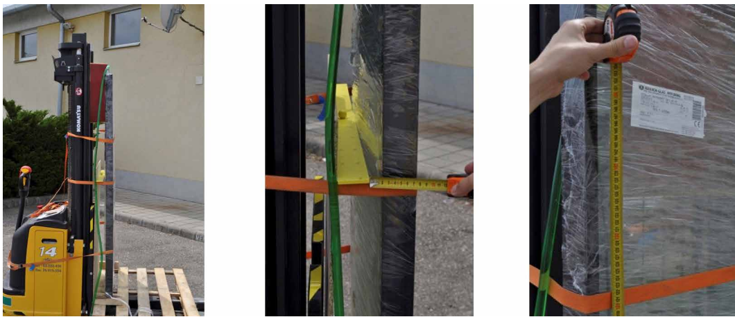
FIG. 12 Deformation of glass pane resulting from water pressure, experiment
