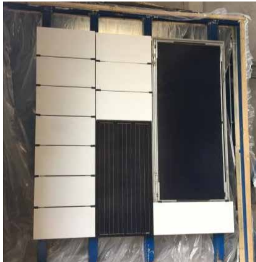
FIG. 11 Performance mock-up of the façade integration, passive (left), PV (centre), and ST (right) claddings
