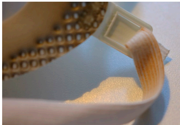
Figure 6. Make-up stains on the polyester elastic from the Alpha Solway respirator.
