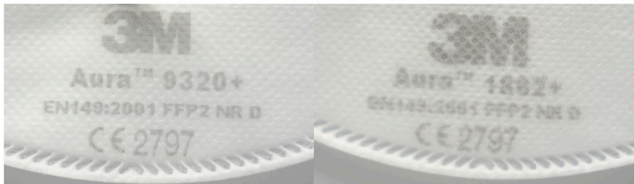
Figure 3. Left: Label of non-sterilised respirator, Right: Blurred label on 3M Aura 1882+ respirator after 1 cycle of steam sterilisation.
