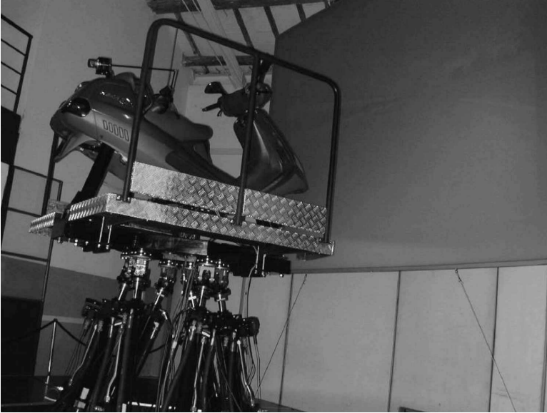
Figure 1.3: Motorcycle riding simulator developed during the MORIS project by the PERCRO Laboratory of the School of Advanced Studies of Pisa [50].
