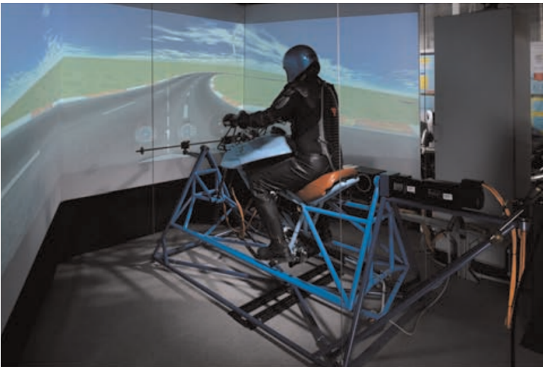
Figure 1.4: Motorcycle riding simulator developed by the University of Padua [32].
