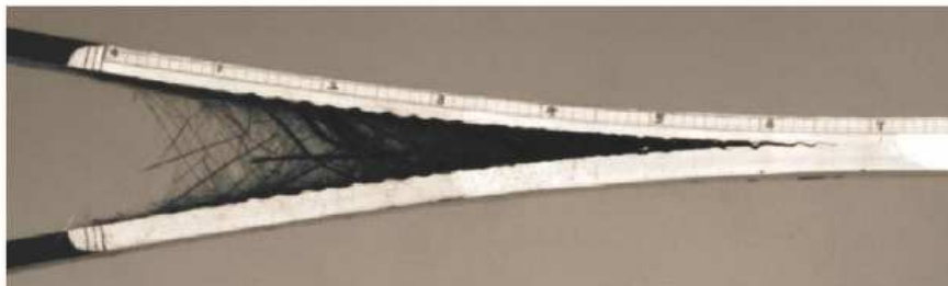
Figure 10 Illustration of delamination growth in a DCB specimen made of carbon fibre polymer composite with fibre bridging as a crack shielding mechanism [70].
