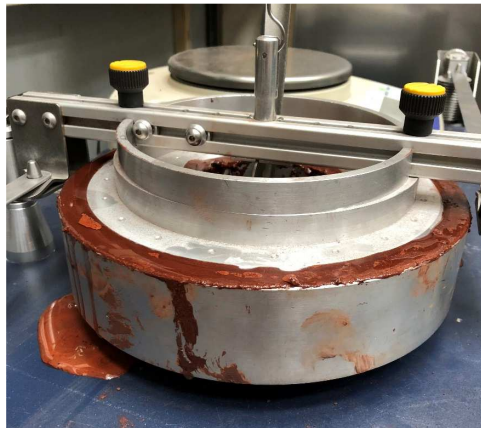
Figure 3-16. Excessive water leaving the sinter feed sample in the wet test condition ( MC_{as,rec+4\%} )
