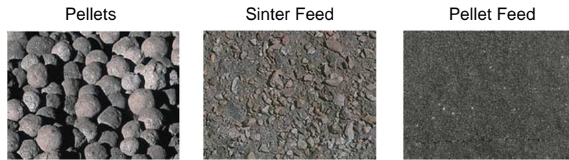
Figure 1-6. Various size range in iron ore products; pellets, sinter feed and pellet feed [21]
