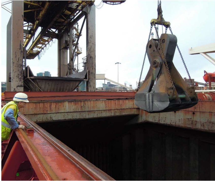
Figure 1-1. Unloading bulk carriers at destination using grabs
