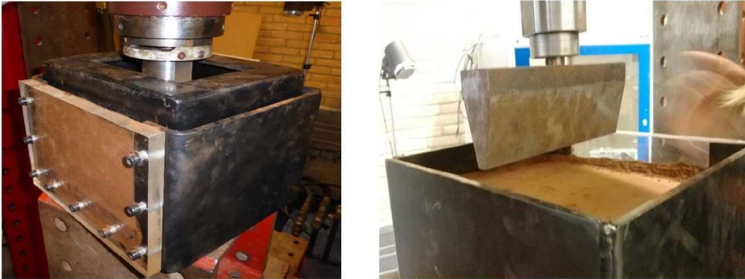
Figure 2-6. Consolidating the iron ore sample; Left) consolidating iron ore with the top plate, Right) Starting point of the penetration phase
