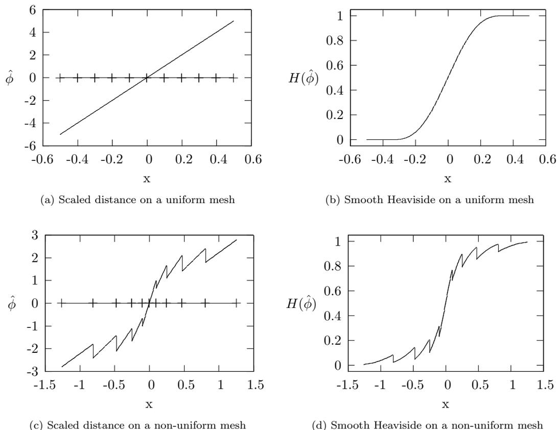
Figure 1: Original scaled distance and smooth Heaviside on a uniform and non-uniform mesh
