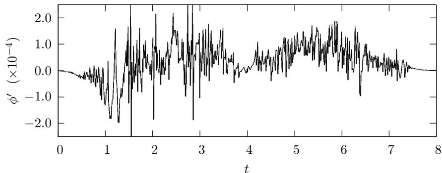
Figure 10: Correction required for volume conservation for the  $80 \times 80$  linear mesh with  $\kappa_d = 1$ .
