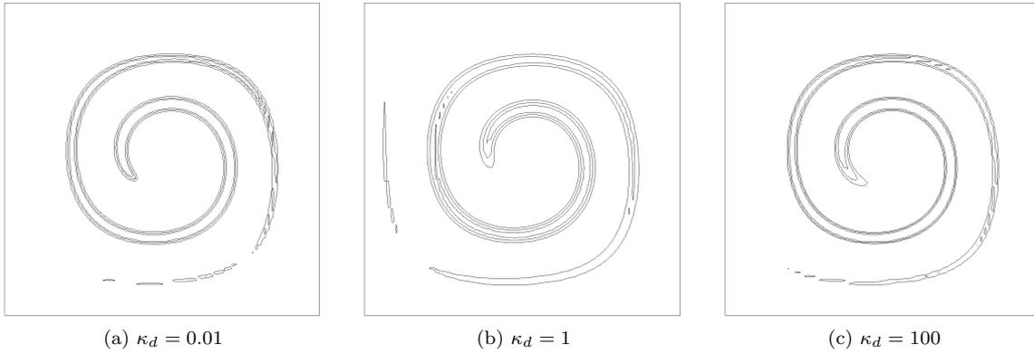
Figure 11: Contour plots of the smooth Heaviside for *projected inverse scaling* on a  $80 \times 80$   $C_0$  linear mesh
