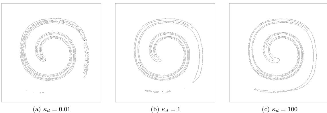
Figure 13: Contour plots of the smooth Heaviside for *projected inverse scaling* on a triangular mesh with 4541 elements
