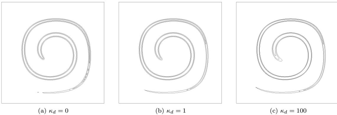
Figure 12: Contour plots of the smooth Heaviside for *projected inverse scaling* on a  $80 \times 80$   $C_1$  quadratic mesh
