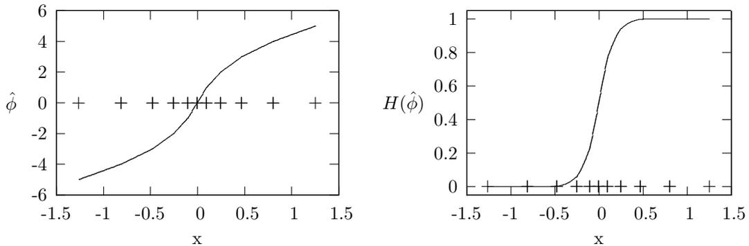
(a) Corrected scaled distance on a non-uniform mesh (b) Corrected smooth Heaviside on a non-uniform mesh
