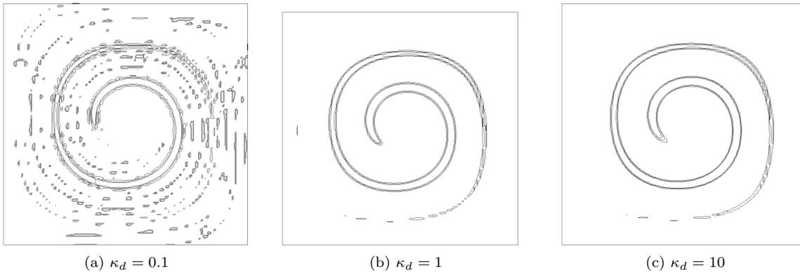
Figure 9: Contour plots of the smooth Heaviside for *projected scaling* on a  $80 \times 80$   $C_0$  linear mesh
