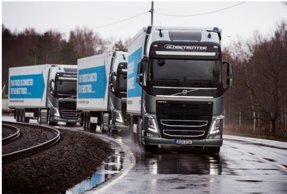
Figure 5: Road Trials of Truck Platoons [27]
