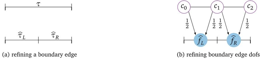
**Fig. 8.** The above depicts refinement of boundary edge dofs. Figure (a) shows the edge labels for the coarse (top) and fine (bottom) meshes. Figure (b) shows how the coarse Bernstein–Bézier form of a spline  $f$  on  $\tau$  (top) can be used to compute the boundary edge dofs for the new boundary edges (bottom).
