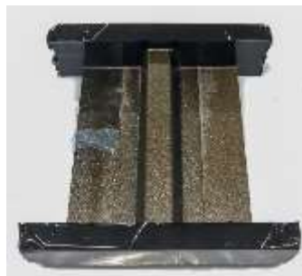
Figure 2. Single-stringer specimens before the test.
