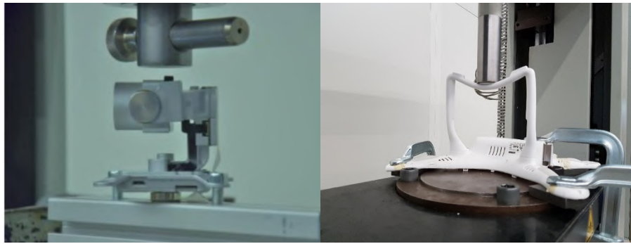
Figure 3.23. Static compressive test to determine the force-deformation curve of each component.
