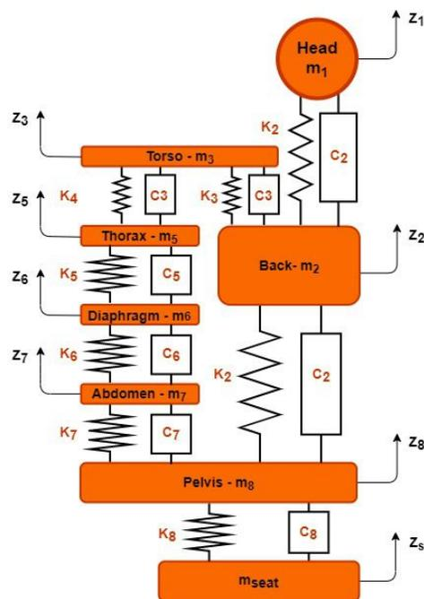
Fig. 4: The biomechanical human body model [16].
