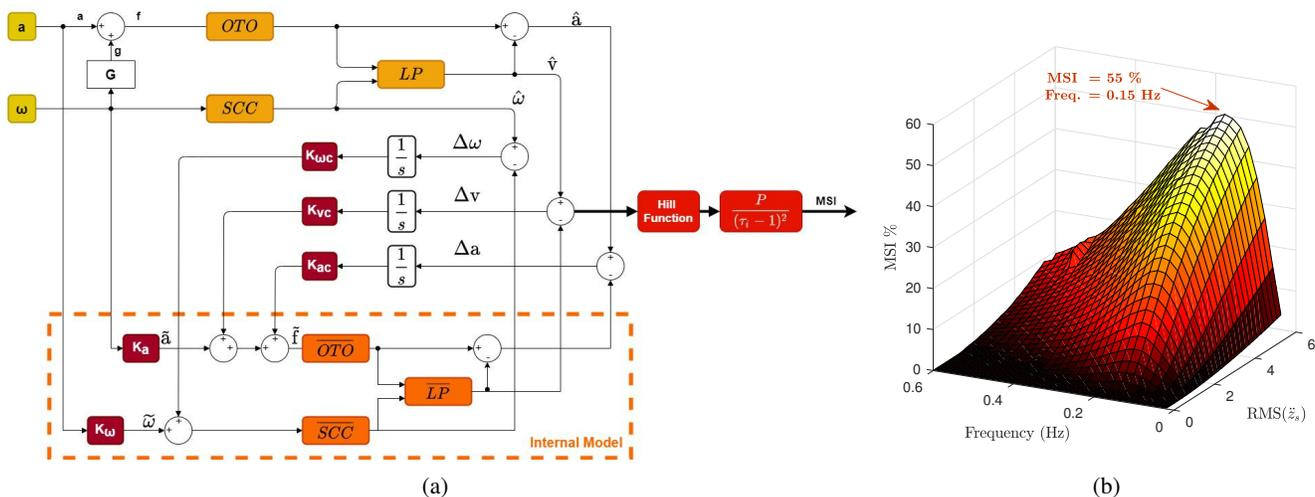
Fig. 3: (a) Six degrees of freedom subjective vertical conflict model, and (b) its validation with regards from Bos et al. [11] and McCauley et al. [12].
