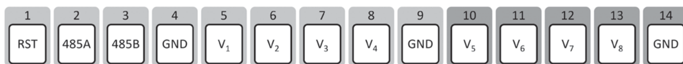
Fig.5 Proposed PQ9 and CS14 electrical interface standards.
