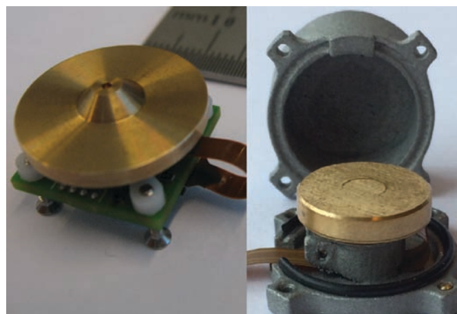
Fig.7 Delfi-n3Xt (left) and Delfi-PQ (right) reaction wheels.
