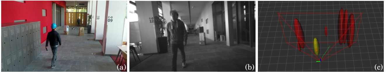
Fig. 7: Results of the experiment Scenario 2. The MAV is flying in a corridor while avoiding static and moving obstacles. (a) A snapshot during the experiment. (b) An on-board grayscale image captured in the experiment and (c) visualization of the corresponding obstacle detection and trajectory planning results.
