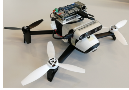
Fig. 4: MAV used in the experiments. It is equipped with an NVIDIA Jetson TX2 Module for all on-board computation, an Intel RealSense Depth Camera D435i dually for visual-inertial odometry and depth image sensing.
