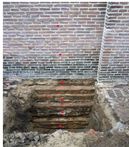
FIG. 3.13 Excavation of the ground around the foundation of the church and sampling, at different depths and heights in the wall along a vertical profile, for the measurement of the moisture content and distribution / Photo: B. Lubelli
