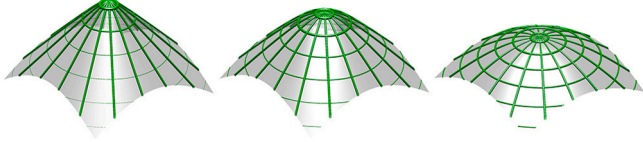
Fig. 5. The multiquadrics is an RBF that has a shape parameter \rho that allows the RBF to take a shape between a cone and a paraboloid as \rho takes a value between 0 and \infty (left to right).
