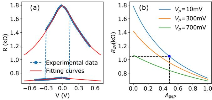
Fig. 9. (a) R-V loop experimental data vs. fitting curves to extract  $R_P$  &  $R_{AP}$  at varying voltage, (b)  $R_{IM}$  vs.  $A_{IMP}$  with respect to three voltages.
