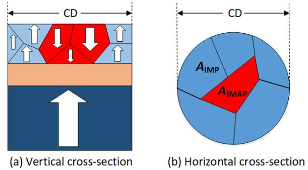
Fig. 7. MTJ schematics with both P-state and AP-state regions in the FL simultaneously.
