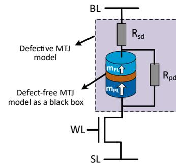
Fig. 6. Resistive models for MTJ-internal defects in the conventional test.
