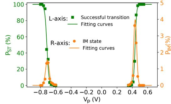
Fig. 10. Curve fitting of  $P_{ST}$  and  $P_{IM}$  to measurement data.
