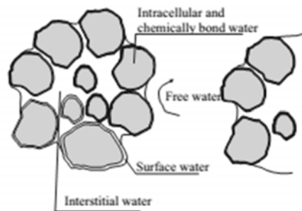
Figure 3: Distribution of water in the sludge floc (Neyens et al., 2003b)
