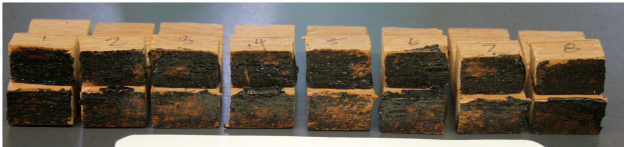
Figure 7. Bonded surfaces after impact test failures. Even presence of tar on upper and lower adherends indicates failures were cohesive in nature.
