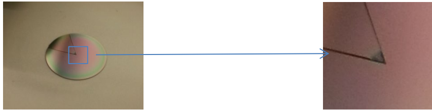
Figure 5.9: Image of the circular Al metal plate in the PECVD machine (left) after deposition of Glass, in the centre the chip is visible (right). In this way we ensure that the plasma ‘sees’ a flat surface.
