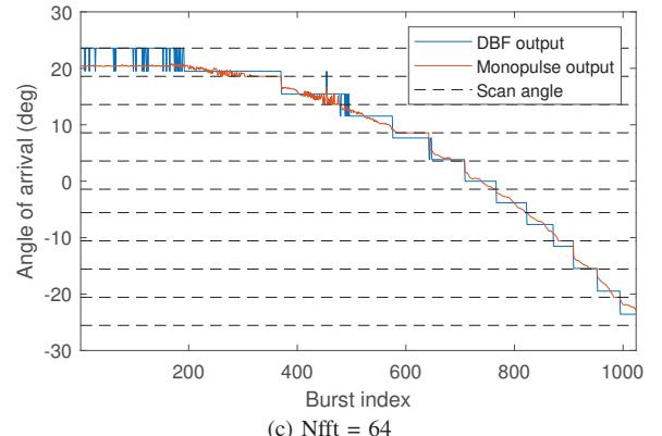
Fig. 3. Result of an indoor experiment single target localization. Blue line is the traditional FFT processing. Red line is the MIMO-Monopulse output. Dashed black lines show the scan angles for realizing monopulse.
