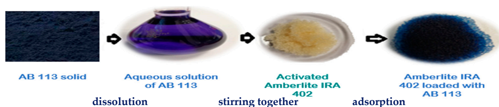
Figure 3. Image of batch adsorption process of AB 113 onto Amberlite IRA 402.
