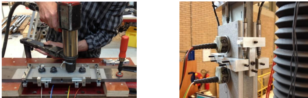
Figure 5.3-2: Application of pretension using air driven torque tool; mounting of LVDT brackets on cover plates
