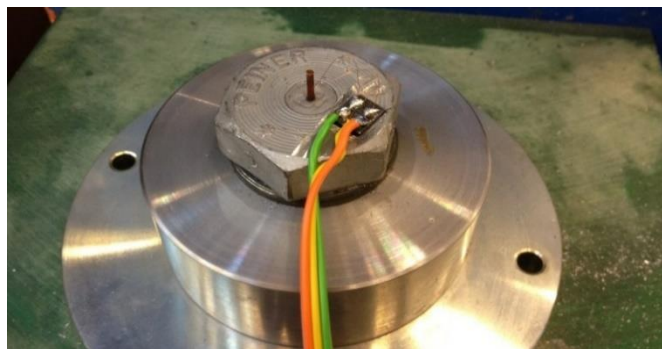
Figure 3.5-2: Strain gauge installed in bolt and connected to terminal. Bolt is placed in Skidmore-Wilhelm instrument.
