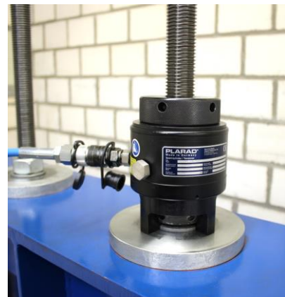
b) tensioner with the capacity of 600 kN
