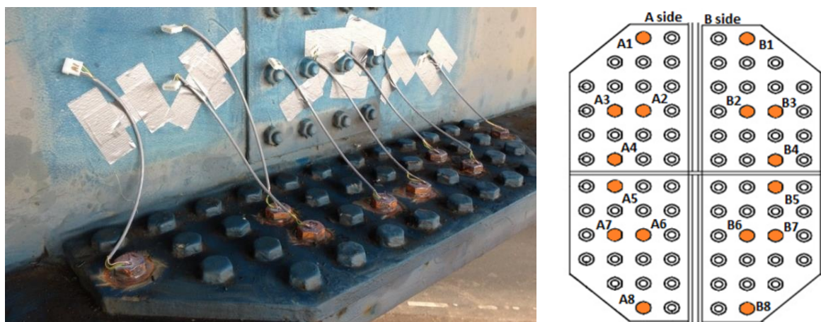
Figure 3.5-3: Instrumented bolts in the beam flange friction grip connection in the Middachterbrug (1974)
