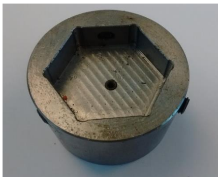
Figure 3.5-1: Hexagonal die used to (1) centre and (2) keep the drill parallel to the bolt axis.
