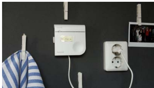
Figure 3.1: Temperature, Relative Humidity and CO 2 sensor box
