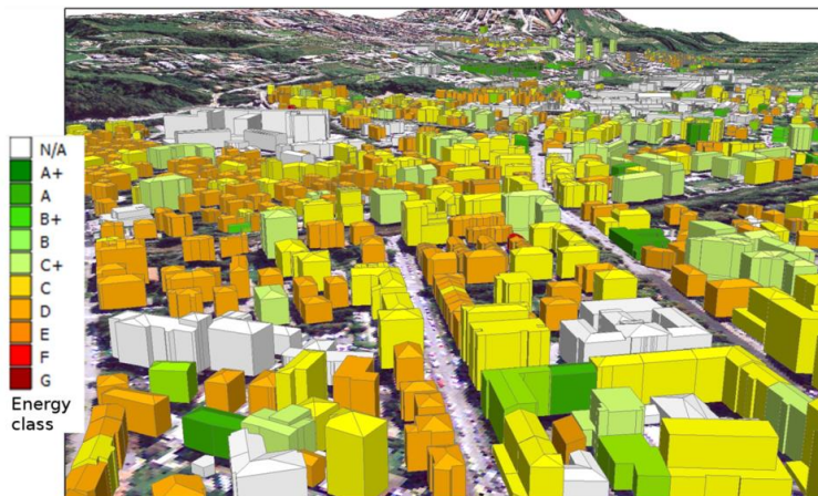
Figure 4: Example of heating energy demand estimation for residential buildings in the city of Trento, Italy. (Source: Agugiaro 2014).
