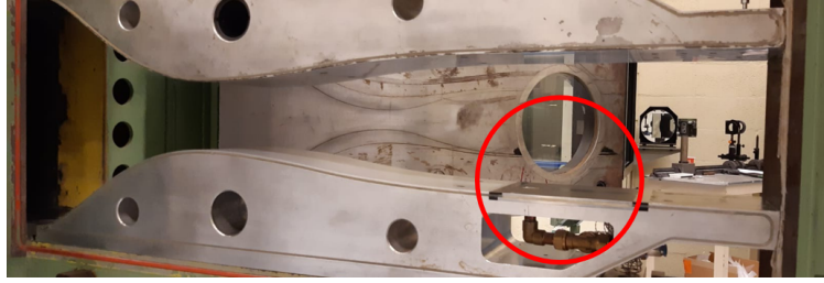
Fig. 1 Test section of the ST-15 supersonic facility. Mach-2 nozzle installed and plate with transverse jet positioned for testing indicated with red circle.
