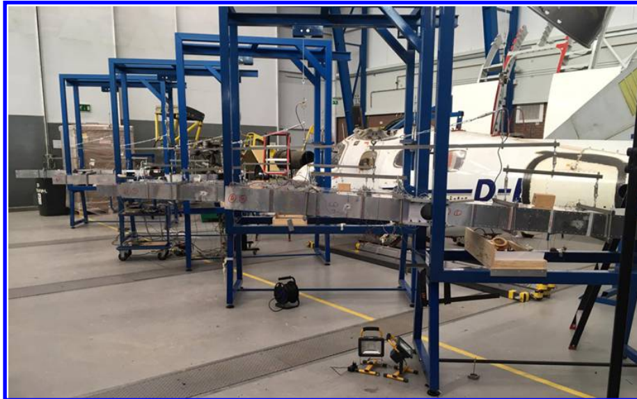
Fig. 4 Five Wing designs in testing rig with distributed load ready to be tested.
