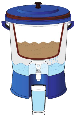
Figure 1-2 Illustration of CPF in use, adapted from WHO (2016) 53
