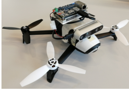
Figure 3.4: MAV used in the experiments. It is equipped with an NVIDIA Jetson TX2 Module for all on-board computation, an Intel RealSense Depth Camera D435i dually for visual-inertial odometry and depth image sensing.
