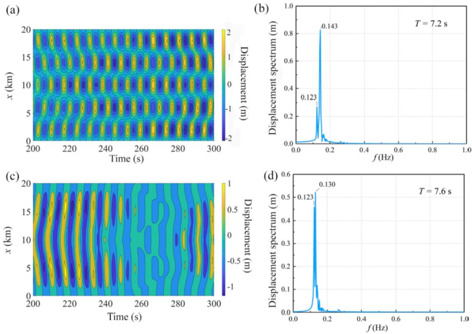
Fig. 20. (a, b) Time series of IL displacement along the entire span, and mid-span frequency spectrum at  $T = 7.2$  s; (c, d) Time series of IL displacement along the entire span, and mid-span frequency spectrum at  $T = 7.6$  s.
