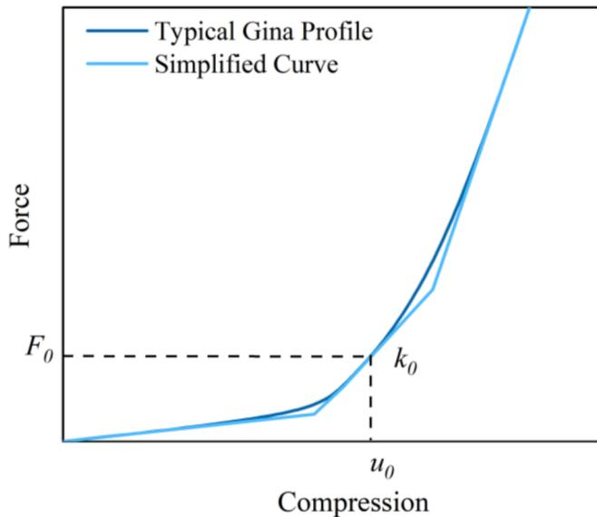
Fig. 6. Gina gasket loading-compressive behavior.
