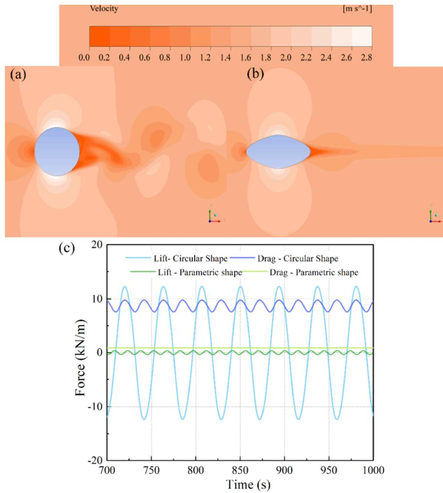
Fig. 14. (a) Instantaneous flow velocity contour for the circular shape; (b) Sequential flow velocity contour for the parametric shape; (c) Drag and lift time-history for the two shapes at  $V = 1.5$  m/s.
