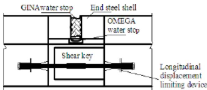
Fig. 7. Schematic drawing of the SFT joint design [43].
