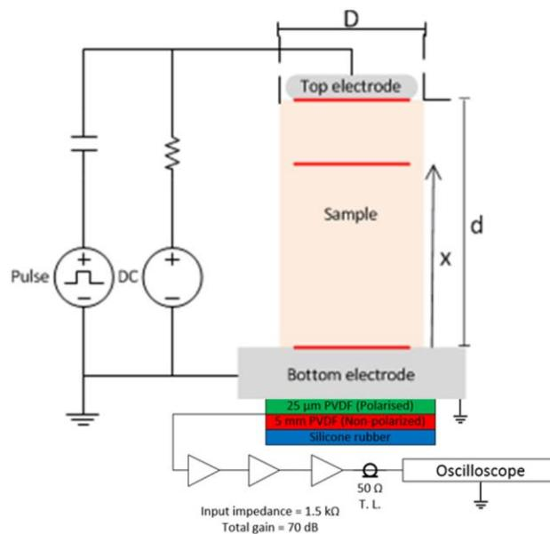
Figure 9. Schematic representation of a PEA measurement for a flat sample. The sample diameter is several times bigger than the height ( $D \gg d$ ), but the scale is modified for representation purposes.
