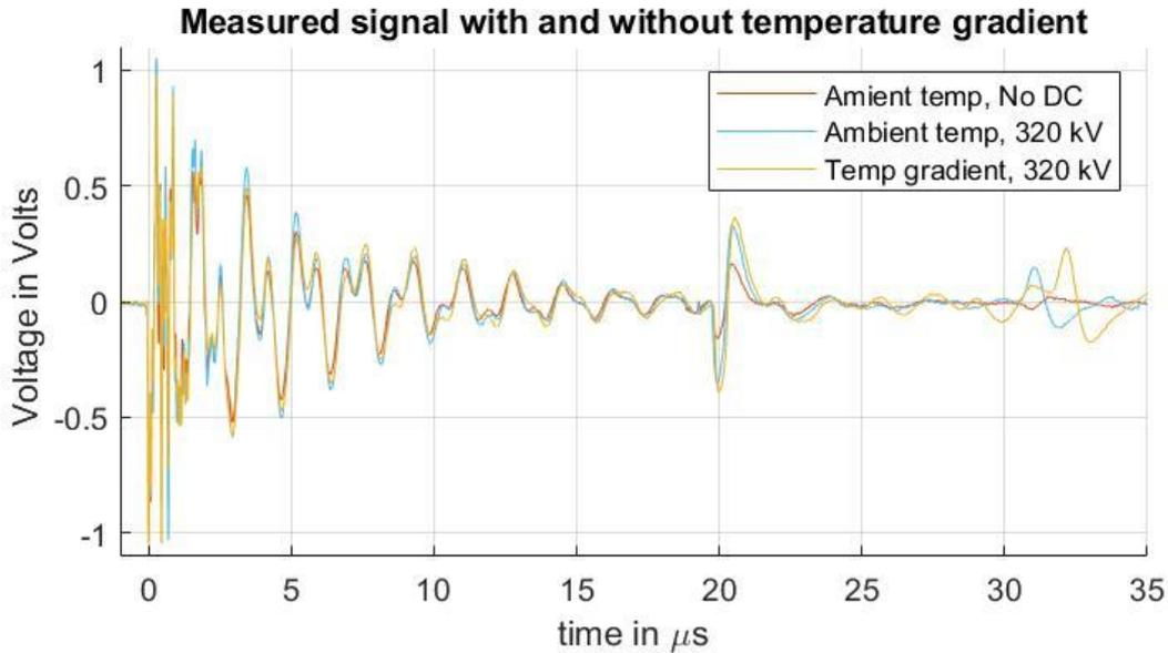
Figure 34. Measured signals at KEMA laboratories for a 320 kV HVDC cable including the measured signals before and after applying 320 kV HVDC without cable heating (no temperature gradient) and the measured after applying 320 kV HVDC after 26.5 hours of cable heating with a temperature gradient of 70° C at the inner conductor and 30° C at the outer conductor.
