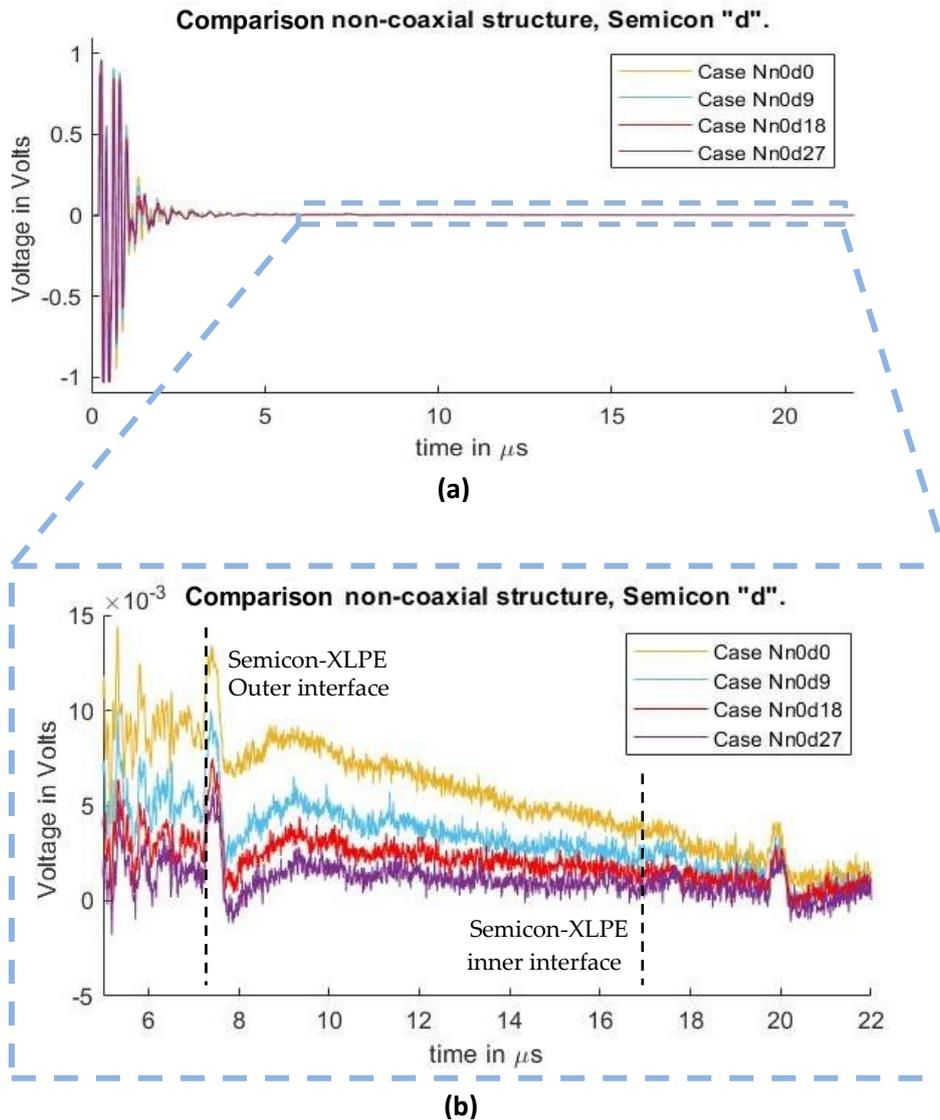
Figure 49. Measured disturbance for Cases with different distances " $d$ " for non-coaxial injection. (a) Full measured signal ranging from the instant of the pulsed voltage application up to 22  $\mu\text{s}$ . (b) Zoom to the time instant of the acoustic signal arrival belonging to the charge measurements.
