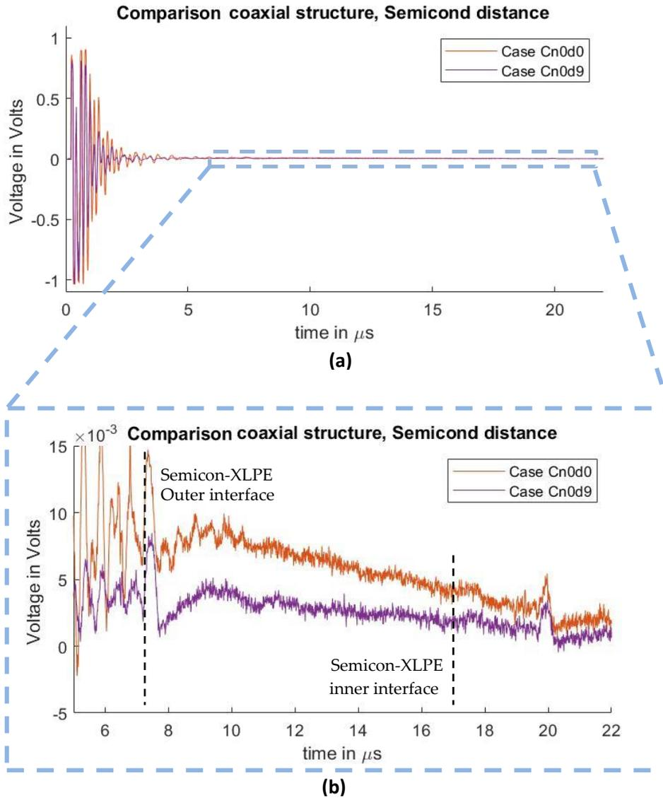
Figure 54. Measured disturbance for Cases with different distances " $d$ " for coaxial injection. (a) Full measured signal ranging from the instant of the pulsed voltage application up to 22  $\mu\text{s}$ . (b) Zoom to the time instant of the acoustic signal arrival belonging to the charge measurements.
