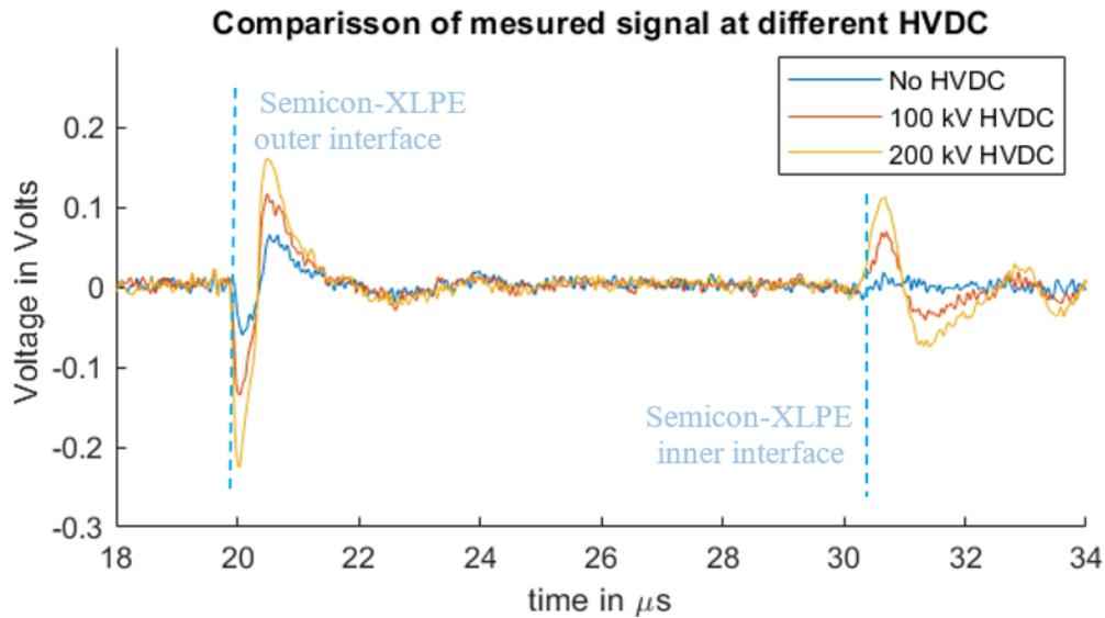
Figure 38. Measured signals with different applied HVDC magnitudes and a 5.5 kV pulsed voltage at the voltage pulse generator.
