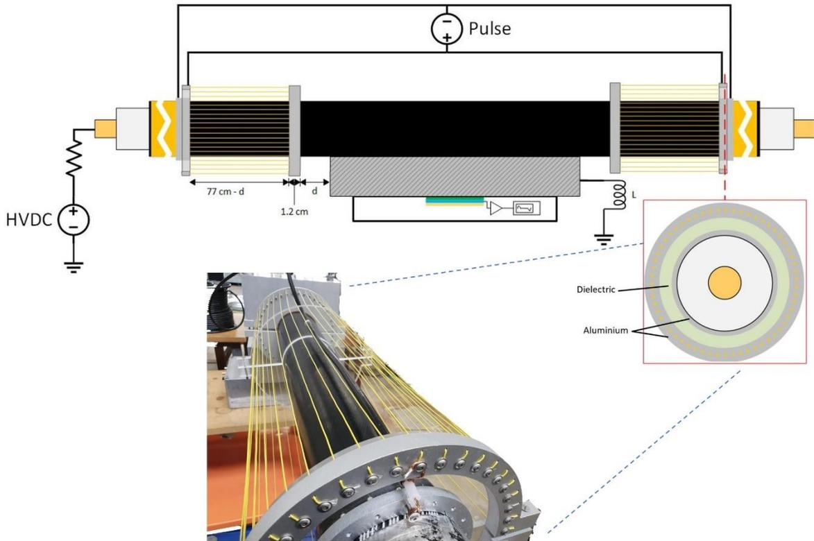
Figure 47. Application of the pulsed voltage at the HVDC test cable using the coaxial configuration. “ $d$ ” stands for the distance between the injection electrode and the PEA test cell, “ $L$ ” is the applied inductance at the PEA test cell grounding.
