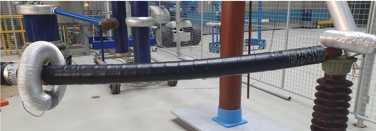
Figure 32. Photo of one of the temporal terminations at the HVDC cable.
