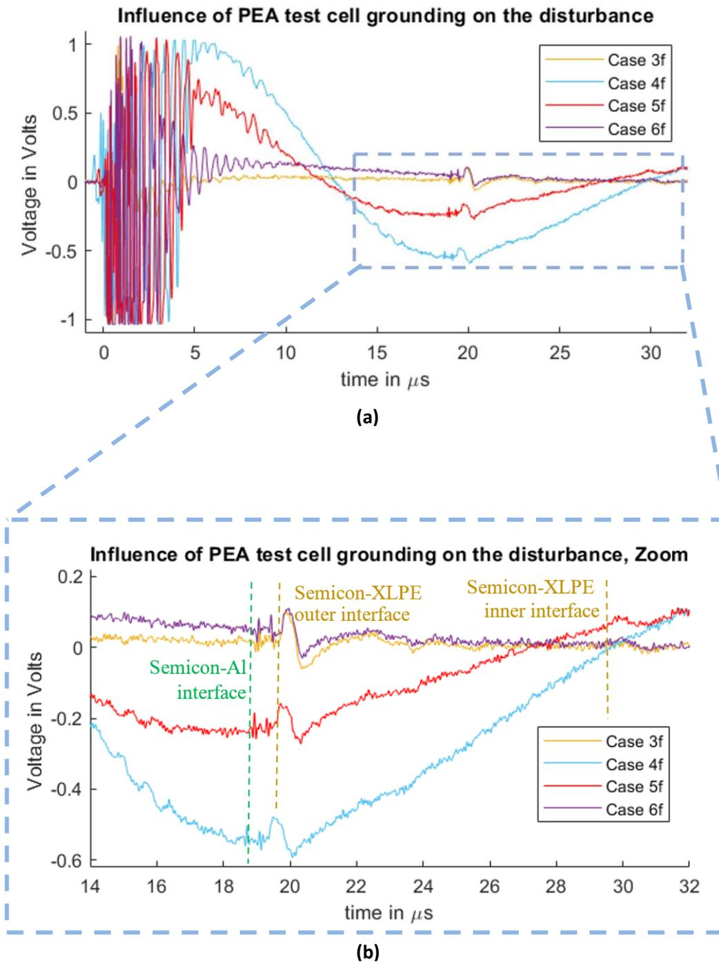
Figure 43. Measured disturbance from Cases 3f, 4f 5f and 6f. (a) Full measured signal ranging from the instant of the pulsed voltage application up to 32  $\mu\text{s}$ . (b) Zoom to the time instant of the acoustic signal arrival belonging to the charge measurements.
