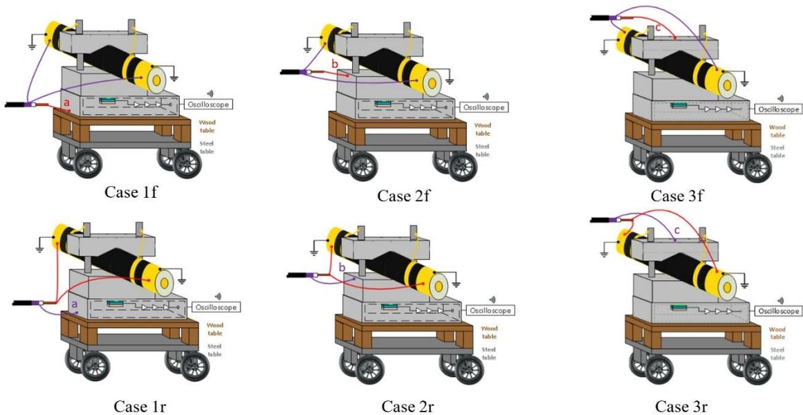
**Figure 39. A 3D representation of the pulsed voltage connection locations for Cases 1f, 1r, 2f, 2r, 3f and 3r. Each of these cases has a different current distribution across the PEA test cell with a different impact in the piezo amplifier interference. The connection between the test cell and the guard is done through the yellow cables at the mechanical pressure screws.**
