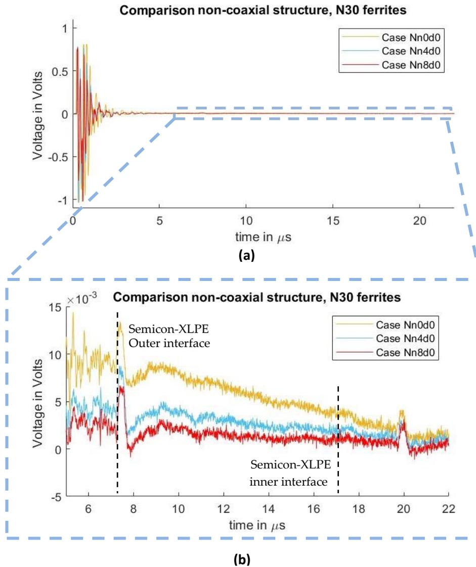
Figure 51. Measured disturbance for cases with different ground inductance “ $L$ ” for non-coaxial injection. (a) Full measured signal ranging from the instant of the pulsed voltage application up to 22  $\mu\text{s}$ . (b) Zoom to the time instant of the acoustic signal arrival belonging to the charge measurements.
