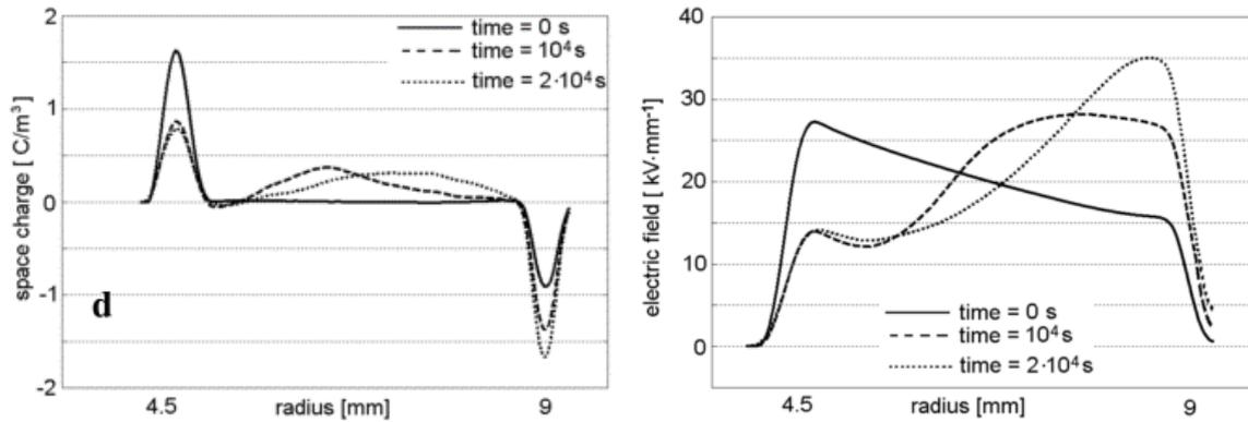
Figure 2. Space charge accumulation and the resultant electric field enhancement [36].
