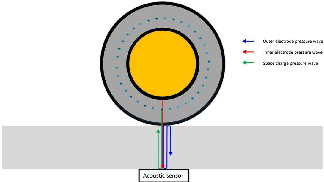
Figure 22. Representation of the acoustic propagation of the pressure waves generated at the inner electrode, outer electrode and at internal space charges for a 21.5 mm dielectric thickness, 1.5 mm outer electrode thickness and 40 mm aluminium base electrode thickness.
