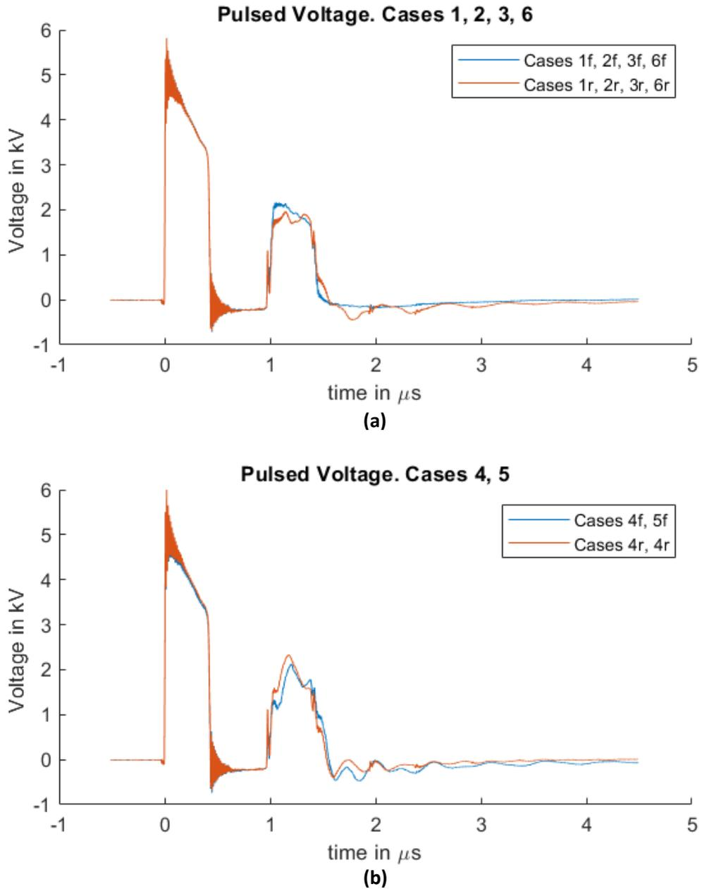
Figure 37. The measured voltage at the voltage pulse generator. The signal from 0 to 0.3  $\mu\text{s}$  belongs to the outgoing pulse; the signal after 0.8  $\mu\text{s}$  is the reflected voltage at the HVDC connection. (a) Measured voltage for cases 1, 2, 3 and 6. (b) Measured voltage for cases 4 and 5.
