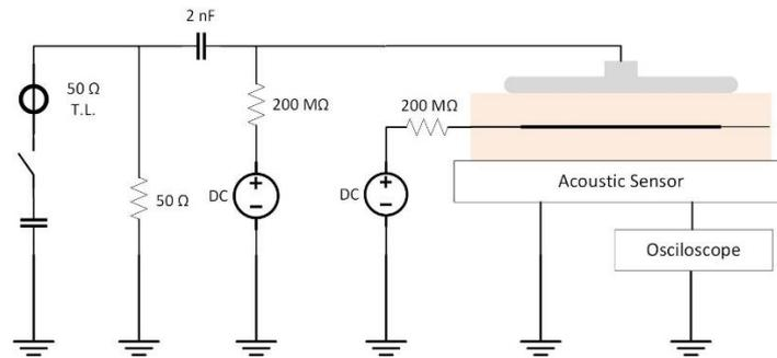
Figure 15. Test setup utilized in the multilayer sample.
