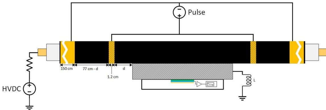
Figure 46. Application of the pulsed voltage at the HVDC test cable using the non-coaxial configuration. “ $d$ ” stands for the distance between the injection electrode and the PEA test cell, “ $L$ ” is the applied inductance at the PEA test cell grounding.
