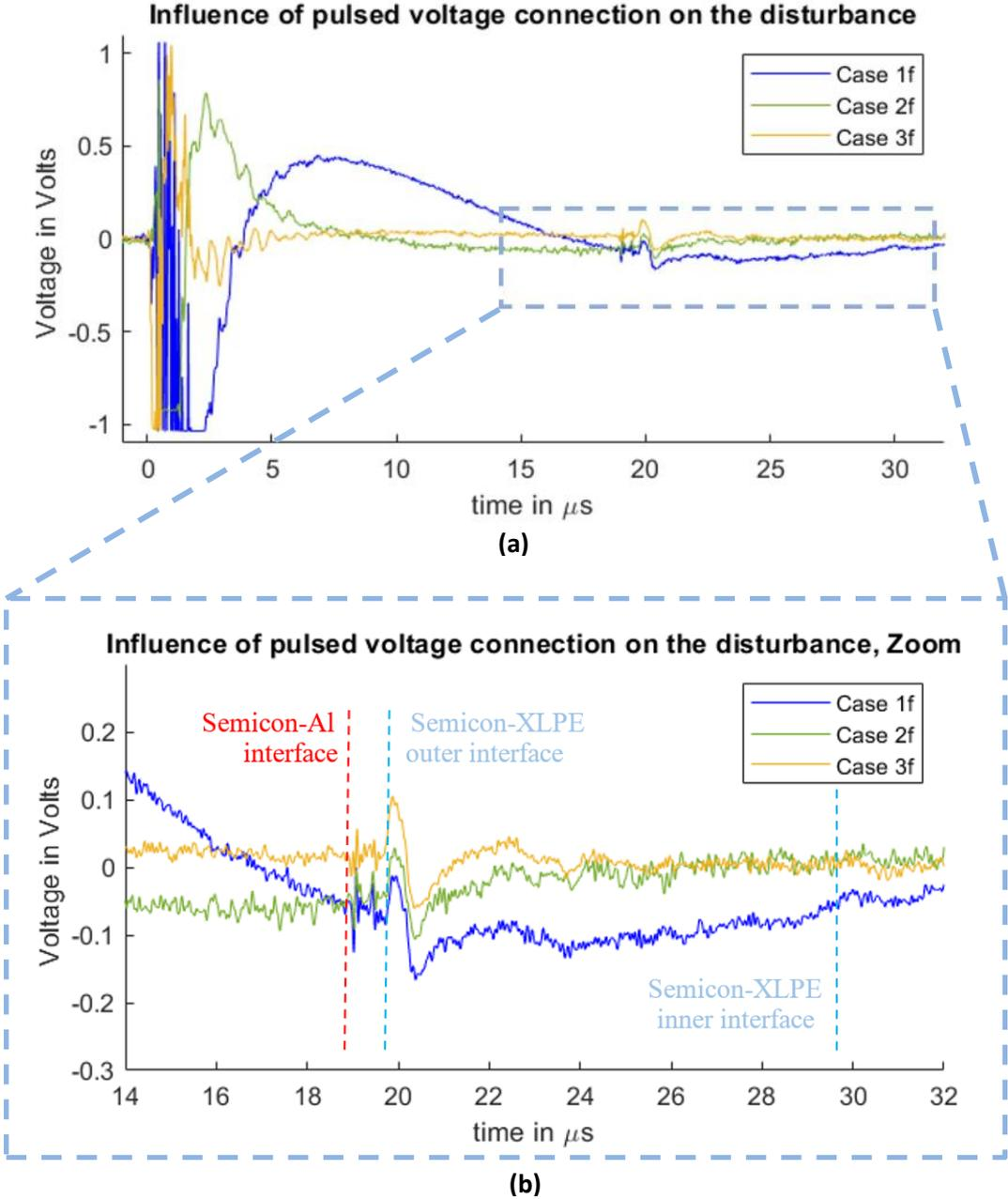
Figure 40. Measured disturbance from Cases 1f, 2f and 3f. (a) Full measured signal ranging from the instant of the pulsed voltage application up to 32  $\mu\text{s}$ . (b) Zoom to the time instant of the acoustic signal arrival belonging to the charge measurements.
