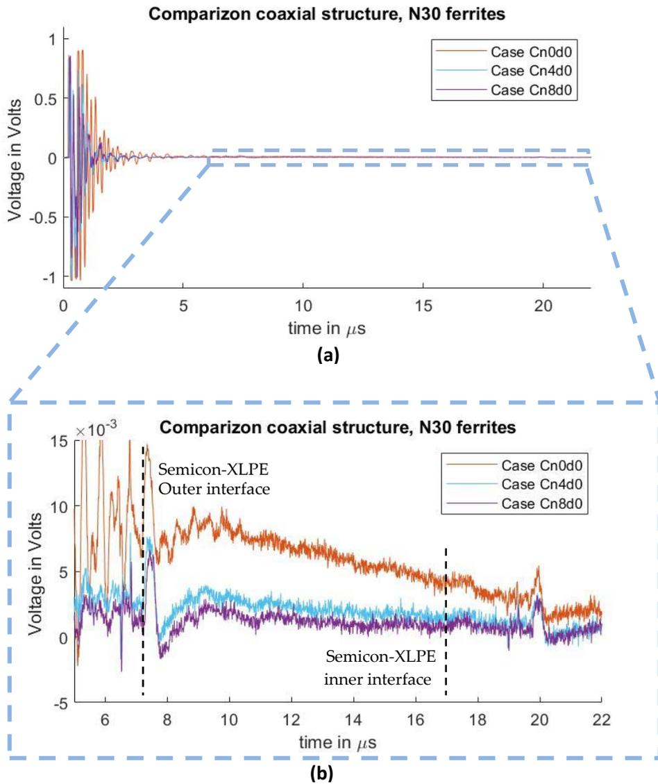
Figure 55. Measured disturbance for cases with different ground inductance “L” for coaxial injection. (a) Full measured signal ranging from the instant of the pulsed voltage application up to 22  $\mu\text{s}$ . (b) Zoom to the time instant of the acoustic signal arrival belonging to the charge measurements.
