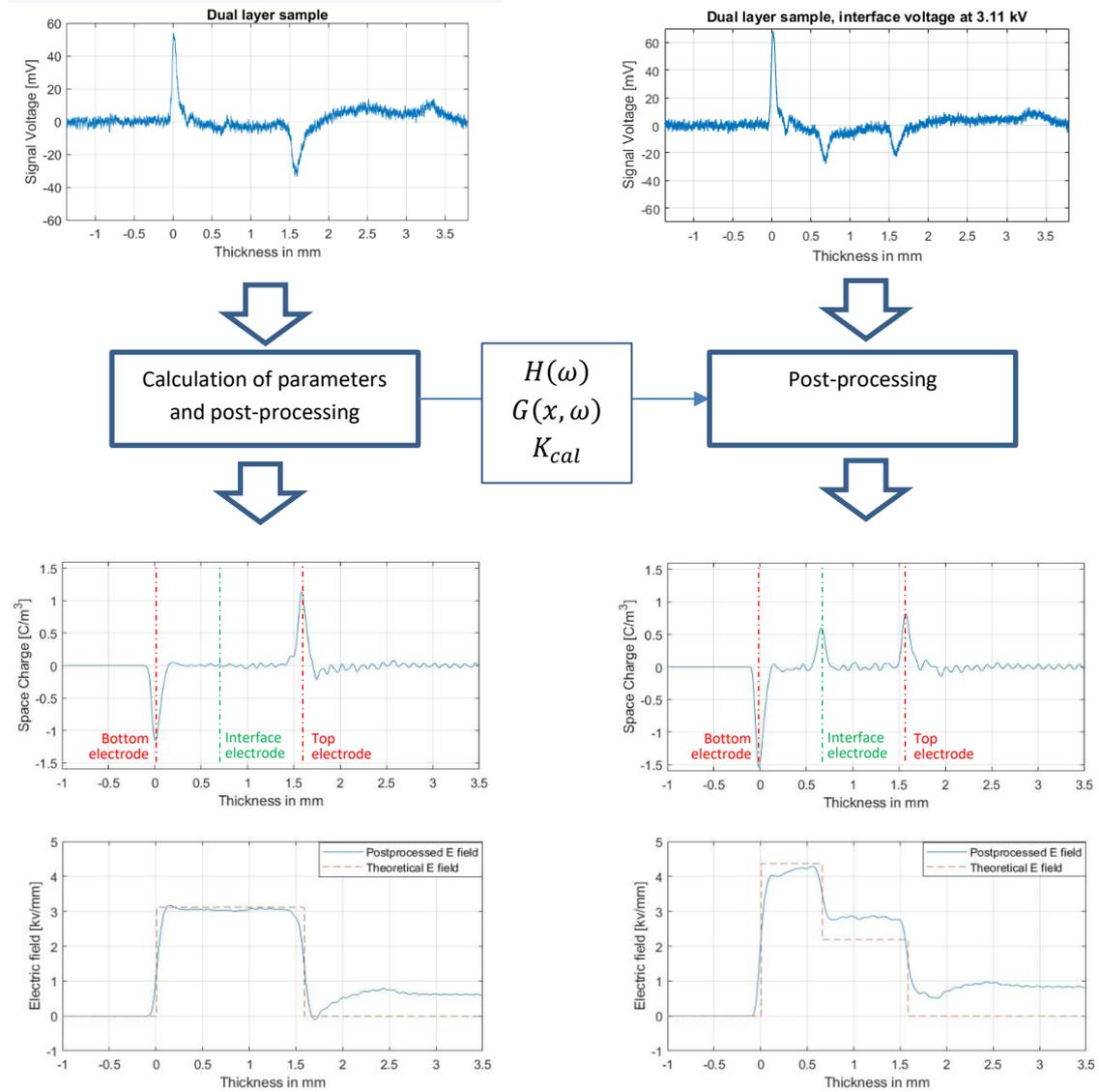
**Figure 20. Postprocessing of Measured values for Space Charge distribution calculations of the dual layer sample with 3.11 kV inner electrode voltage, using the measured signal with 2.14 kV inner electrode voltage to calculate the post-processing parameters.**
