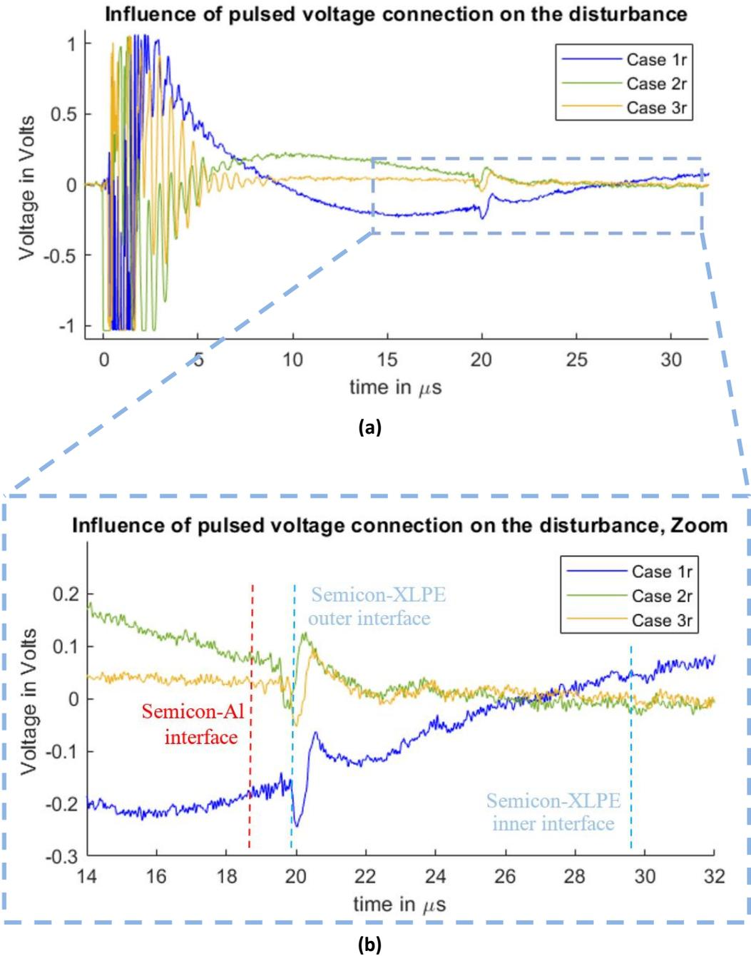
Figure 41. Measured disturbance from Cases 12, 2r and 3r. (a) Full measured signal ranging from the instant of the pulsed voltage application up to 32  $\mu\text{s}$ . (b) Zoom to the time instant of the acoustic signal arrival belonging to the charge measurements.
