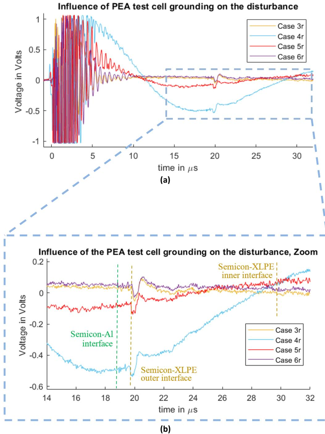
Figure 44. Measured disturbance from cases 3r, 4r, 5r and 6r. (a) Full measured signal ranging from the instant of the pulsed voltage application up to 32  $\mu\text{s}$ . (b) Zoom to the time instant of the acoustic signal arrival belonging to the charge measurements.
