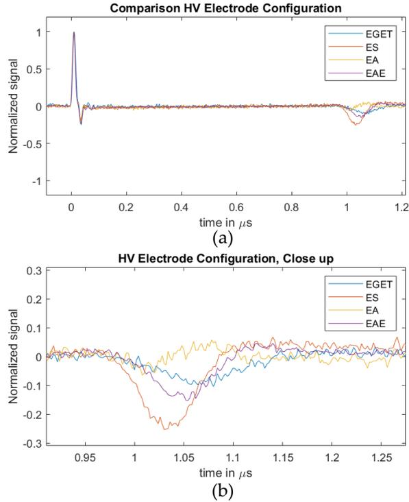
Figure 10. Normalized PEA measurement Samples 1 and 2 at 10 kV: (a) Full signal, (b) Close up at the HV electrode.
