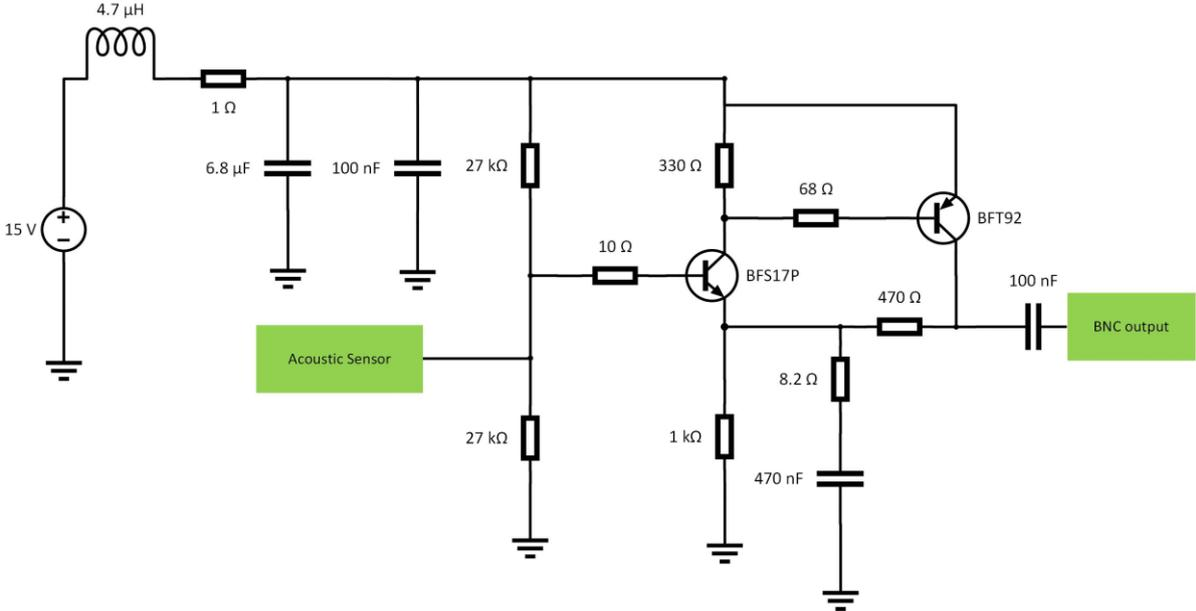
Figure 24. Charge amplifier equivalent circuit diagram.
