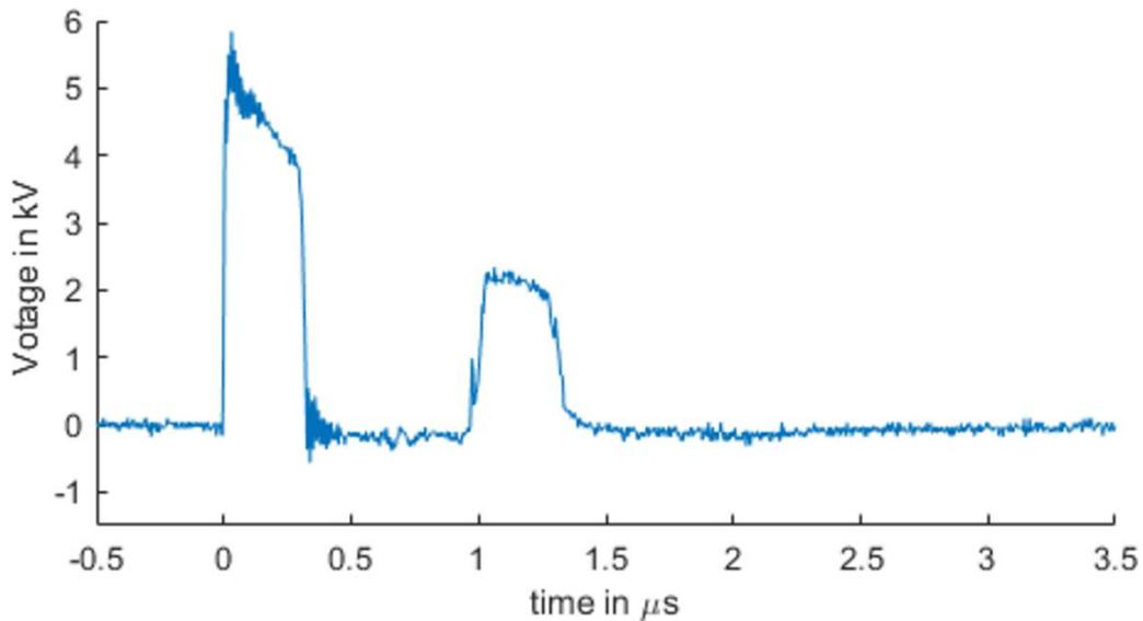
Figure 29. Measured voltage at the pulsed voltage generator. The signal from 0 to 0.3  $\mu\text{s}$  belongs to the outgoing pulse; the signal after 0.9  $\mu\text{s}$  is the reflected voltage at the HVDC connection.
