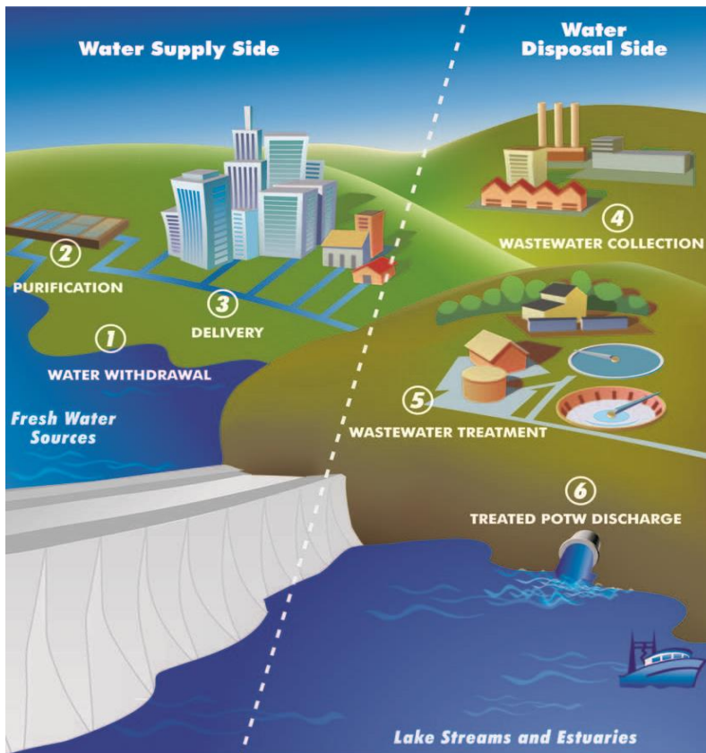
Figure 2: simplified urban water cycle (POTW is the abbreviation of publicly owned treatment works) (EPA, 2004)
