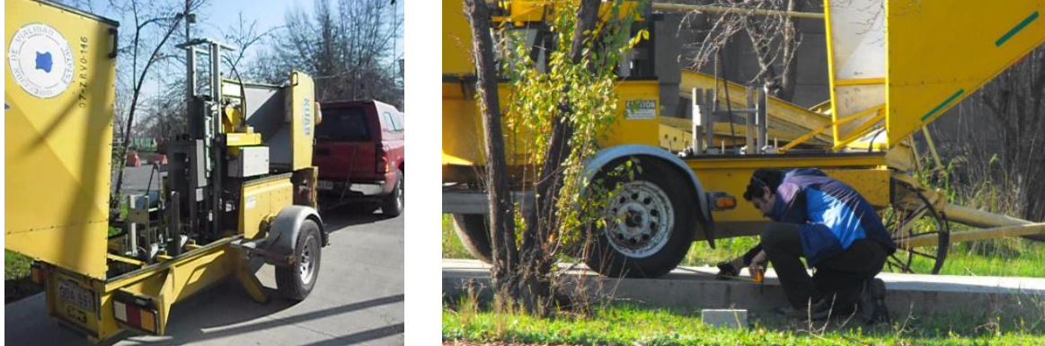
Fig 6.5.3. Application of load repetitions with the FWD on an uncracked joint
