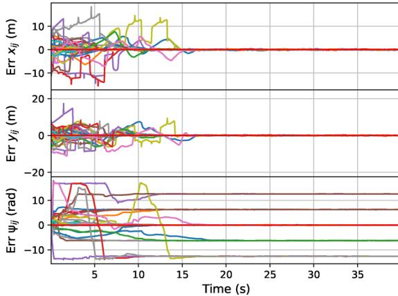
**Figure 5.** 30 simulation experiments of the optimal controller with random initial MAV positions. This figure shows the estimation errors of 2-axis relative positions and 1-axis relative orientation.
