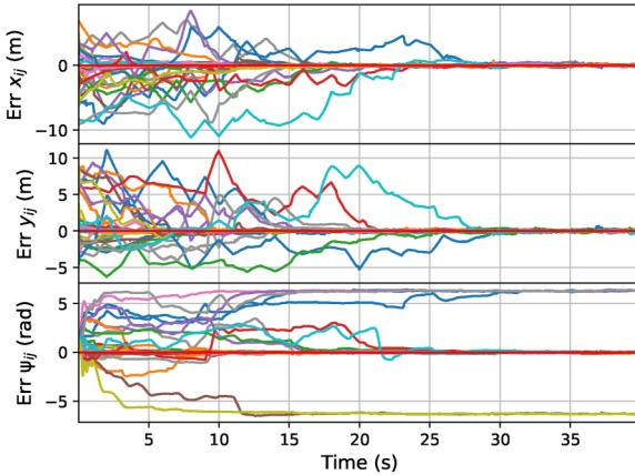
**Figure 4.** 30 simulation experiments of the stochastic controller from<sup>16</sup> with random initial MAV positions. This figure shows the estimation errors of 2-axis relative positions and 1-axis relative orientation. Note that yaw error with  $-2\pi$  or  $2\pi$  offset has no influence on the relative localization due to the cos and sin operation.
