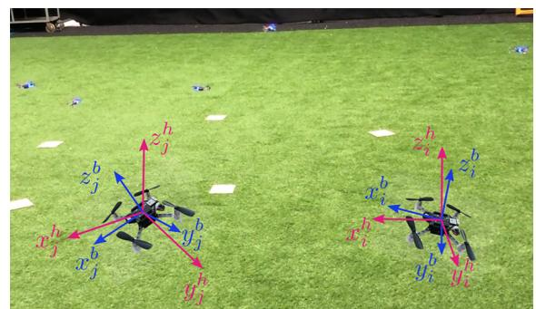
**Figure 1.** The diagram of a twin-MAV kinematic model, and two coordinated frames. Body frames and horizontal frames are shown with blue axes and red axes, respectively. Both frames are fixed to the robot, while the horizontal frames always have a vertical Z-axis. The background image shows previous experiments of multi-MAV relative localization but without optimal control.
