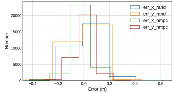
**Figure 7.** Localization error of two controllers after estimation convergence. Each distribution has a total of 15000 data points on these 30 random tests, which is taken from the last 5 seconds when all estimators have converged.
