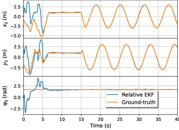
**Figure 9.** Relative localization and ground-truth between two MAVs under the proposed optimal control method and formation tracking multi-robot tasks. The target relative position is constant before  $t = 15$ s, and variant after  $t = 15$ s.
