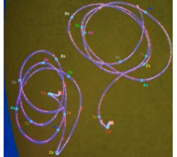
**Figure 11.** The optimal motion trajectories of two Crazyflies under the proposed NMPC controller. On each trajectory, ten stars are representing the drone position with respect to time after take-off at 0s.
