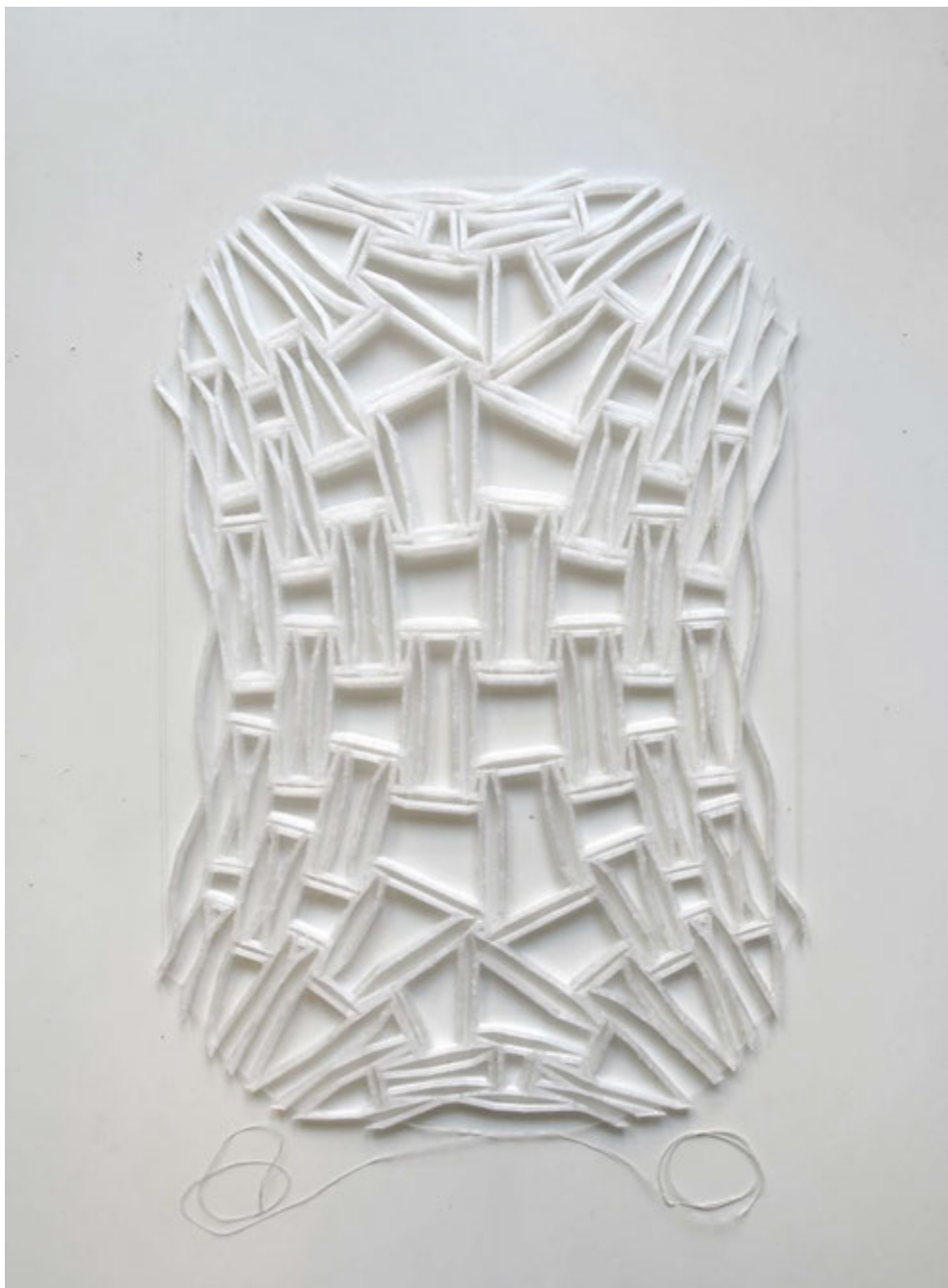
Figure 6.15: Flat configuration of the free-edge shell
