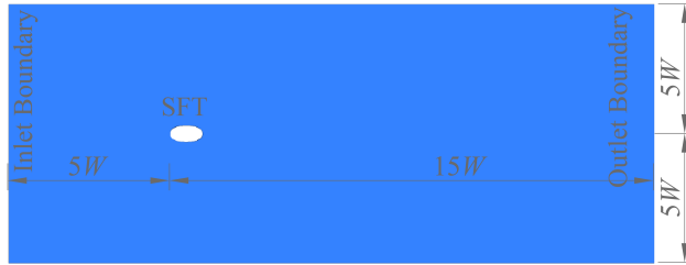
Figure 2.5: Schematic diagram of the computational domain, W is width of the SFT cross-section
