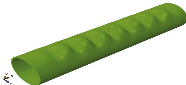
Fig. 4. The initial imperfection in terms of wave-type on pipe surface (imperfection amplitude has been zooming out for the sake of clarity).
