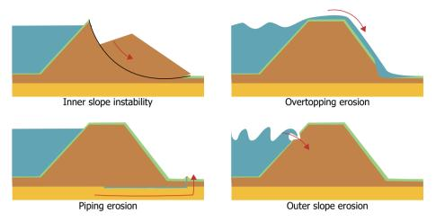
Figure 2.2.: The 4 failure modes considered in this thesis. More information can be found in concerning chapters and the International Levee Handbook [3].
