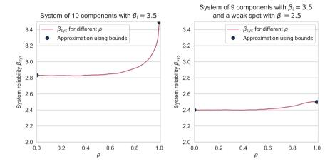
Figure 2.4.: System reliability for a system of 10 elements. Left pane: all elements have  $\beta_i = 3.5$ . Right pane: one element has  $\beta_i = 2.5$ .
