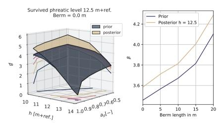
Figure 4.3.: (left) Prior and posterior fragility surface (in terms of reliability index  $\beta$ ) of the water level h and response factor  $a_p$ , for the considered case study without berm. The overall reliability index (integrated with the prior probability density of  $a_p$  and h) is 3.46. (right) Relationship between berm length and overall reliability index  $\beta$  for the prior situation and posterior after a proof load level of 12.5 m+ref.
