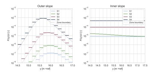
Figure 7.8.: Failure probability  $P_f(y|s)$  for external erosion at the outer (left) and inner (right) slope (with  $s \in S$ ). Dotted coloured lines indicate  $P_f(y|s)$ , solid lines indicate the discrete values per zone z along the slope. Values are for a single flood defence section.
