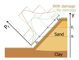
Figure 7.3.: Failure probability along the slope for 2 states s with (brown) and without (green) damage. Solid lines indicate  $P_{\rm f}(y|s)$ , dashed lines indicate the probability of failure for a slope part  $P_{\rm f}(z|s)$ .
