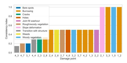
Figure 6.8.: Consistency index of different damage points with more than 3 registrations in the database. Colors indicate the reference classification parameter (see Table 6.1) except for 'Transition' where no reference parameter could be determined, and burrowing where small and large burrows are combined.
