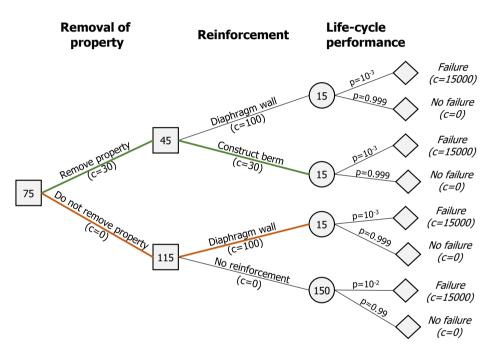
Figure 2.9.: Decision tree for a reinforcement decision. The decision has 2 choice nodes (squares): a choice to remove adjacent property, and a choice of a reinforcement method. Values in the nodes indicate the total cost of the optimal decisions conditional on the choice in that node.
