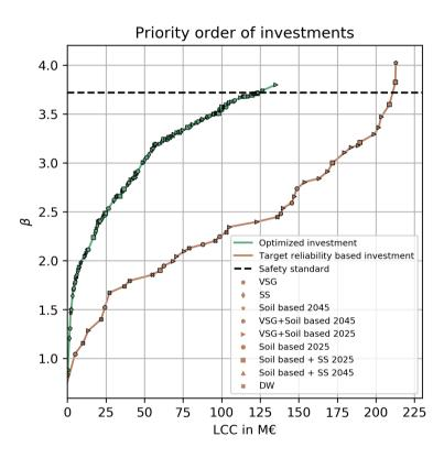
Figure 3.6.: Priority order for optimized investments (green) and investments based on target reliability (brown). Markers denote different types of measures at different dike sections,  $\beta$  is the reliability index in 2075.
