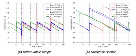
Figure 5.2.: Two calculations of  $\beta$  in time for samples  $x_i \in \mathbf{x}_n$  for Case B. The left pane shows an unfavourable sample ( $\beta_{\text{state}} > \beta_{\text{belief}}$ ). The right pane a favourable sample. Circled markers on the line for strategy b indicate presence of monitoring equipment. Dotted vertical lines indicate a reinforcement.
