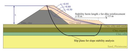
Figure 4.2.: Cross section of the considered case study. Blue lines indicate the simplified schematization of the phreatic line for different response factors  $a_{\rm p}$  (at an extreme water level).
