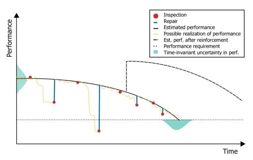
Figure 1.1.: Schematic representation of life-cycle performance. Black line denotes the performance as typically considered for long term investments, whereas the yellow line shows a possible realization such as dealt with in inspection (red dots) and maintenance (repairs represented by blue vertical lines). Life-cycle performance is also subject to time-invariant uncertainty (green distribution). In time, opportunities might arise for reinforcement (black dashed line).
