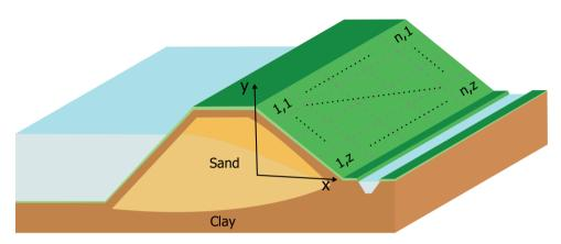
Figure 7.1.: Schematized flood defence segment consisting of n sections (1 km length). The slope of each section is divided into z zones at which occurrence and consequences of damages are considered. The flood defence consists of a clay cover layer with grass revetment and a sandy core.
