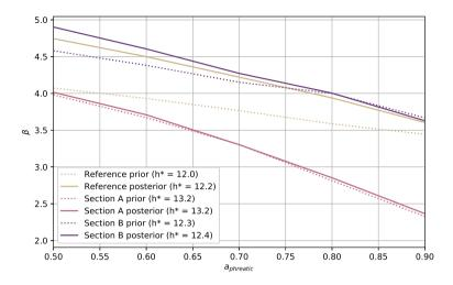
Figure 4.8.: Fragility curves at the design point water level, showing an increasing dependency for the response factor  $a_{\text{p(hreatic)}}$  after proof loading (steeper curve).
