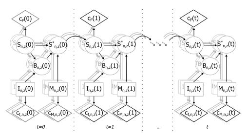
Figure 7.5.: Influence diagram for inspections I, maintenance M and state development S of dike section n and slope zone z including different cost contributions at every time step. Note that shaded nodes and edges represent different sections n and slope zones z, which together determine the  $c_F(t)$  (i.e., the cost of failure of the system).
