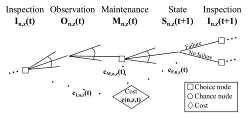
Figure 7.4.: Generic decision tree for the sequential actions of inspection, observation, maintenance and state development of dike section n and slope zone z.
