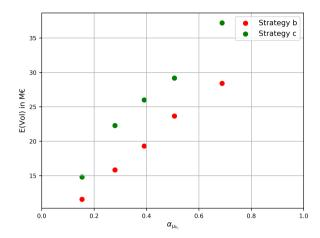
Figure 5.4.: Relation between the influence coefficient of the strength  $\alpha_{\mu_{h_c}}$  and the expected Value of Information (VoI).
