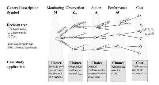
Figure 4.10.: Decision tree for the second case. Note that monitoring can only be done at 1 section, and that the set of actions **A** denotes all reinforcement measures for the entire dike segment.
