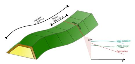
Figure 3.1.: Relation between dike segment, dike section and cross section and schematic representation of the reliability in time for a single cross section for different failure modes as considered in this chapter.
