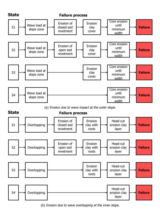
Figure 7.2.: Failure processes for both failure modes for different states of the revetment.
