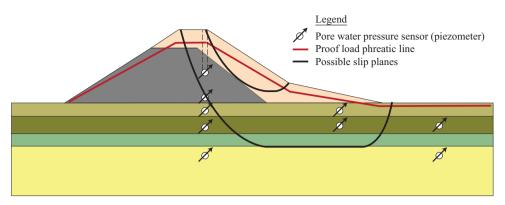
Figure 4.4.: Overview of the positioning of sensors installed for pore water pressure monitoring, and the imposed phreatic level during a proof load test. The larger black line indicates the slip plane relevant for flooding, the smaller slip plane is relevant for failure of the proof load test but does not cause flooding.
