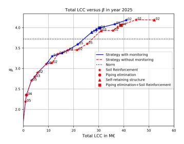
Figure 4.14.: Total investment costs (LCC) versus the reliability for the entire segment for prioritized investments with and without monitoring for a scenario with  $P(k_{\rm repr}) = 0.025$ . Symbols indicate different measures, numbers indicate the section. Where lines overlap identical measures are taken in both strategies.
