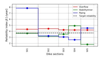
Figure 4.11.: Reliability indices  $\beta$  for each section per failure mode in 2025. The dashed black line denotes the target reliability for the segment as a whole.
