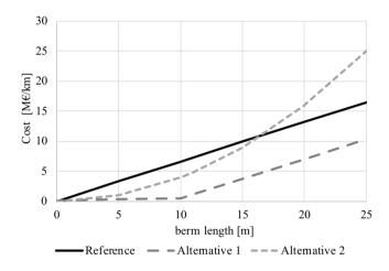
Figure 4.5.: Different cost functions for dike reinforcements.
