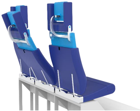
Figure 7: the top recline mechanism
