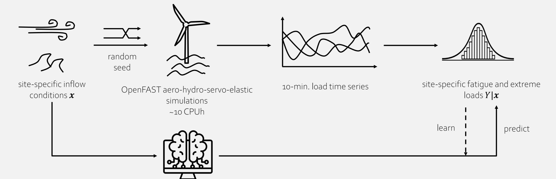
probabilistic surrogate model (lowcost approximation of the system) ~1 CPUs
