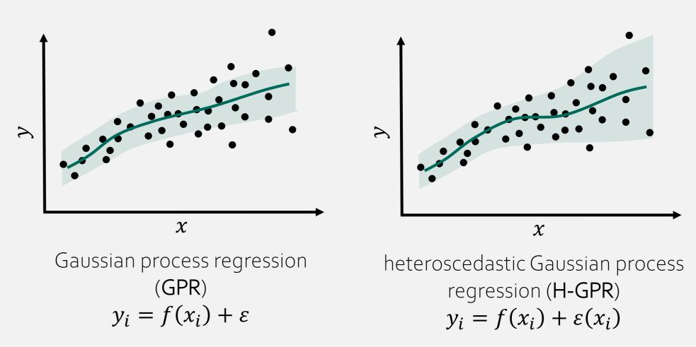
Bayesian statistical methods like the heteroscedastic Gaussian process regression can directly infer the underlying mean and variance of the pdf from a noisy database.
