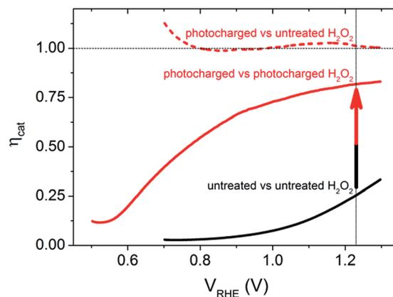
Fig. 2 Calculated catalytic efficiency for the untreated (black solid curve) and photocharged  $\text{BiVO}_4$  samples (red curves). The catalytic efficiency for the photocharged samples was estimated using the  $JV$  characteristics in the presence of  $\text{H}_2\text{O}_2$  for the untreated sample (dashed red curve) and with the photocharged sample (solid red curve).
