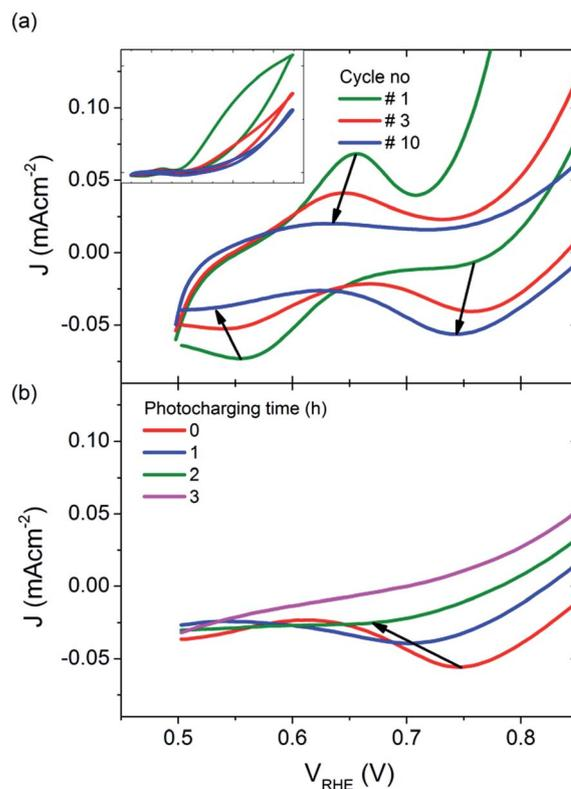
Fig. 6 *JV* scans under illumination, for (a) untreated BiVO<sub>4</sub>, inset: full potential range, and (b) BiVO<sub>4</sub> photocharged for different periods of time (cathodic sweeps only).
