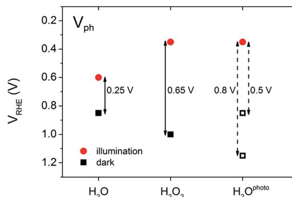
Fig. 4 Equilibrium potentials and photovoltage values of BiVO<sub>4</sub> photoanodes in the open circuit configuration: untreated sample in 0.1 M K–Pi electrolyte (H<sub>2</sub>O), in presence of a hole scavenger (H<sub>2</sub>O<sub>2</sub>), photocharged sample (H<sub>2</sub>O<sup>photo</sup>).
