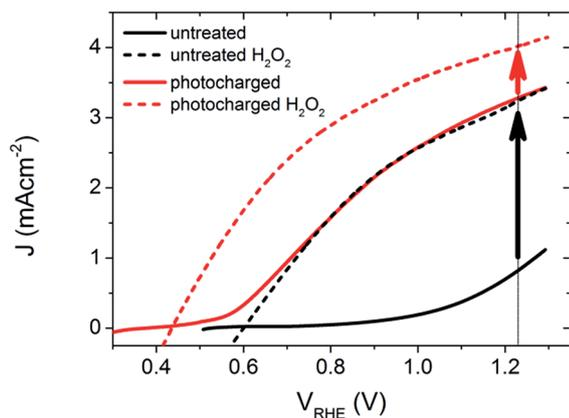
Fig. 1  $J$ - $V$  scans of 200 nm thick  $\text{BiVO}_4$  under back-side AM 1.5 illumination, in 0.1 M K-Pi buffer (pH 7.2), scan rate  $50 \text{ mV s}^{-1}$ , anodic sweeps. Arrows denote catalytic limitations for untreated (black) and photocharged (red) material.
