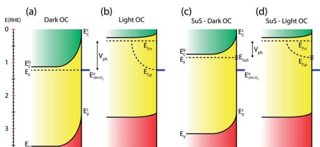
Fig. 3 Estimated electronic band diagrams for BiVO<sub>4</sub> in the OC configuration without surface states present (a) in the dark and (b) under illumination, and with surface states present (c) in the dark, and (d) under illumination.
