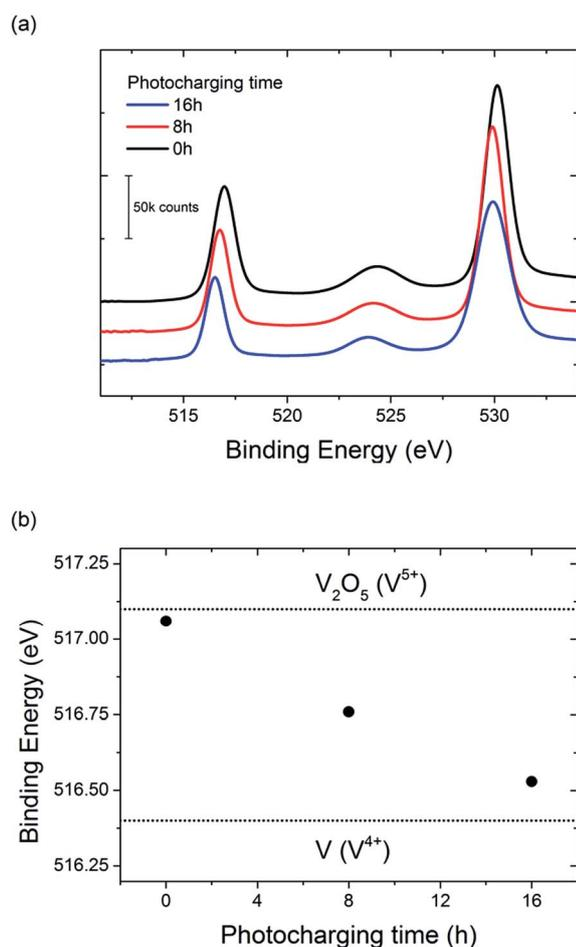
Fig. 7 (a) XPS spectra for BiVO<sub>4</sub> photoanodes photocharged for 0 (black), 8 (red) and 16 h (blue) in K–Pi buffer pH 7.2. (b) V2p<sub>3/2</sub> peak position for BiVO<sub>4</sub> samples photocharged for different amount of time. V<sub>2</sub>O<sub>5</sub> and V(IV) binding energies are shown for reference.
