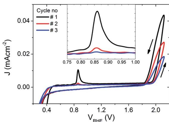
Fig. 5 The first three dark *JV* scans of the BiVO<sub>4</sub> photoanode after 10 hours of photocharging, inset: a zoomed in plot around the observed oxidation peak at ~0.85 V<sub>RHE</sub>.
