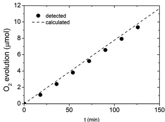
Fig. 8 Gas chromatography detection of O<sub>2</sub> evolved at photocharged BiVO<sub>4</sub> electrode at constant current of 0.65 mA cm<sup>-2</sup>.
