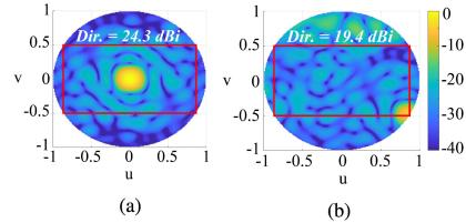
Fig. 11. Radiation pattern (normalized w.r.t. broadside gain, in dB) of the 64-element array optimized for  $p = 1, 2$ . (a) Broadside. (b) Corner beam.
