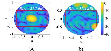
Fig. 15. Radiation pattern (normalized w.r.t. broadside gain, in dB) of the 36-element subset optimized for  $p = 1, 2$ , and 3. (a) Broadside. (b) Corner beam.
