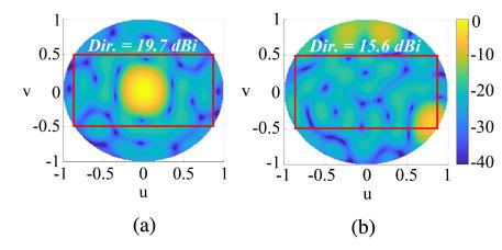
Fig. 16. Radiation pattern (normalized w.r.t. broadside gain, in dB) of the 24-element subset optimized for  $p = 1, 2$ , and 3. (a) Broadside. (b) Corner beam.
