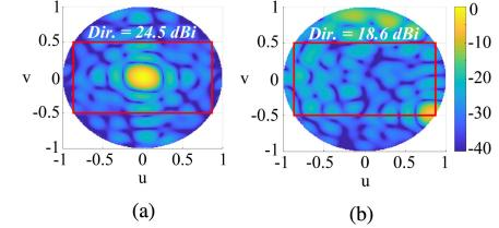
Fig. 14. Radiation pattern (normalized w.r.t. broadside gain, in dB) of the 64-element array optimized for  $p = 1, 2$ , and 3. (a) Broadside. (b) Corner beam.
