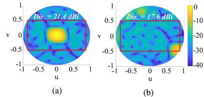
Fig. 12. Radiation pattern (normalized w.r.t. broadside gain, in dB) of the 36-element subset optimized for  $p = 1, 2$ . (a) Broadside. (b) corner beam.
