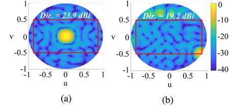
Fig. 5. Radiation pattern (normalized w.r.t. broadside gain, in dB) of the 64-element array optimized for  $p = 1$ . (a) Broadside beam. (b) Corner beam.
